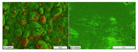
Fig. 3 EDX mapping of the elemental composition of KIT-Z80PU (left) and KIT-Z80AE (right) with aluminum in orange and silica in green.
