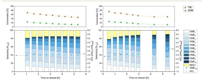
Fig. 6 Experimental results from continuous OME synthesis with KIT-Z80PU (left) and KIT-Z80AE (right) employing feed C2. Reaction conditions: T = 100 °C, p = 40 bar.
