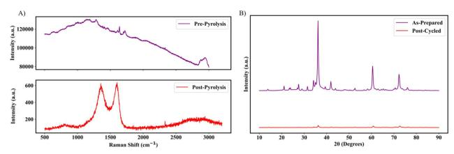
Fig. 3 (A) Raman spectra of the pure transparent red resin before and after pyrolysis, and (B) XRD result of samples pyrolyzed at 1400 °C.
