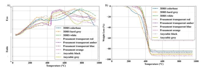
Fig. 2 (A) DTA, and (B) TGA results from different acrylate resins.
