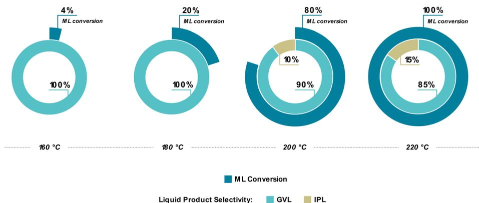
Fig. 7 Effect of reaction temperature on ML conversion and product selectivity for Al<sub>2</sub>O<sub>3</sub>-ZrO<sub>2</sub>/C (1 : 1) under transfer hydrogenolysis conditions (reaction conditions: 0.5 mL min<sup>-1</sup> flow rate; ML 0.2 M in 2-propanol; 0.500 g of catalyst; 30 bar pressure; time on stream: 30 min).
