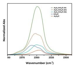
Fig. 2 In situ IR spectra of  $CO_2$  adsorbed on all the pure and mixed oxides recorded at beam temperature. The spectra are corrected for the pellet thickness and focus on the 2400–2300 cm<sup>-1</sup> range, relative to linear  $CO_2$  complexes.
