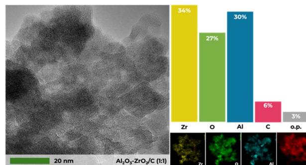
Fig. 5 STEM image and EDX analysis of the Al<sub>2</sub>O<sub>3</sub>–ZrO<sub>2</sub>/C (1 : 1) catalyst.
