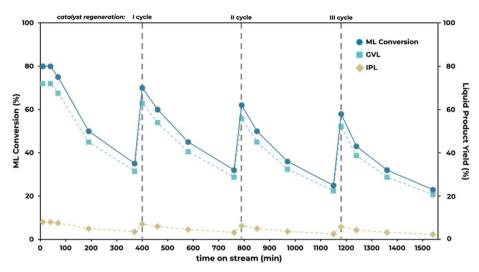
Fig. 8 CTH of methyl levulinate into  $\gamma$ -valerolactone promoted by the Al<sub>2</sub>O<sub>3</sub>-ZrO<sub>2</sub>/C (1:1) catalyst against time (reaction conditions: 0.5 mL min<sup>-1</sup> flow rate; ML 0.2 M in 2-propanol; 0.500 g of catalyst; 30 bar pressure; reaction temperature: 200 °C). The regeneration of the catalyst was performed for three consecutive cycles after 360 min of time-on-stream (dotted gray line).
