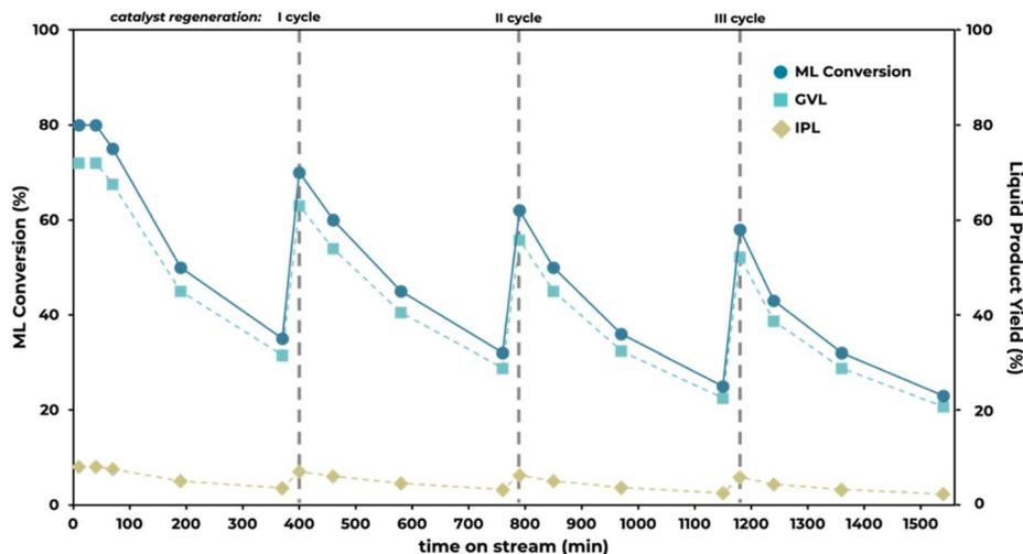
Fig. 8 CTH of methyl levulinate into  $\gamma$ -valerolactone promoted by the  $\text{Al}_2\text{O}_3\text{-ZrO}_2/\text{C}$  (1 : 1) catalyst against time (reaction conditions: 0.5  $\text{mL min}^{-1}$  flow rate; ML 0.2 M in 2-propanol; 0.500 g of catalyst; 30 bar pressure; reaction temperature: 200 °C). The regeneration of the catalyst was performed for three consecutive cycles after 360 min of time-on-stream (dotted gray line).
