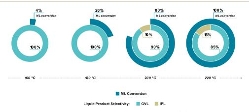
Fig. 7 Effect of reaction temperature on ML conversion and product selectivity for  $Al_2O_3-ZrO_2/C$  (1:1) under transfer hydrogenolysis conditions (reaction conditions: 0.5 mL min<sup>-1</sup> flow rate; ML 0.2 M in 2-propanol; 0.500 g of catalyst; 30 bar pressure; time on stream: 30 min).
