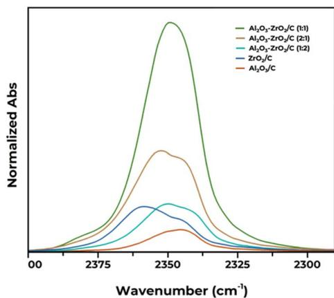
Fig. 2 *In situ* IR spectra of CO<sub>2</sub> adsorbed on all the pure and mixed oxides recorded at beam temperature. The spectra are corrected for the pellet thickness and focus on the 2400–2300 cm<sup>-1</sup> range, relative to linear CO<sub>2</sub> complexes.
