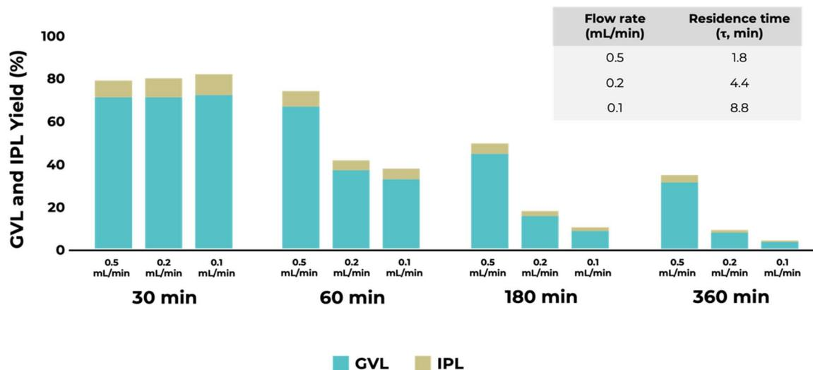
Fig. 9 CTH of methyl levulinate into g-valerolactone promoted by  $\text{Al}_2\text{O}_3\text{-ZrO}_2/\text{C}$  (1 : 1) under a flow rate effect at different times on stream (reaction conditions: ML 0.2 M in 2-propanol; 0.500 g of catalyst; 30 bar pressure; reaction temperature: 200 °C).
