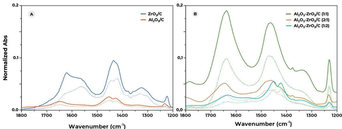
Fig. 4 IR spectra of CO<sub>2</sub> adsorption of pure oxides (A) and mixed oxides (B) with the solid lines corresponding to stabilization of 25 mbar CO<sub>2</sub> and dotted lines to CO<sub>2</sub> outgassing ( $5 \times 10^{-5}$  mbar).
