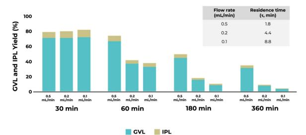
Fig. 9 CTH of methyl levulinate into g-valerolactone promoted by  $Al_2O_3$ – $ZrO_2/C$  (1:1) under a flow rate effect at different times on stream (reaction conditions: ML 0.2 M in 2-propanol; 0.500 g of catalyst; 30 bar pressure; reaction temperature: 200 °C).
