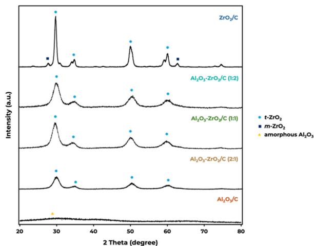
Fig. 1 XRD patterns of calcined MOF-derived  $\text{Al}_2\text{O}_3\text{-ZrO}_2/\text{C}$  catalysts.
