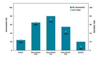
Fig. 6 Catalyst screening in the CTH of methyl levulinate into g-valerolactone promoted by MOF-derived  $Al_2O_3$ – $ZrO_2/C$  catalysts by using 2-propanol as an H-source (reaction conditions: 0.5 mL min<sup>-1</sup> flow rate; ML 0.2 M in 2-propanol; 0.500 g of catalyst; 30 bar pressure; time on stream: 30 min; reaction temperature: 200 °C).
