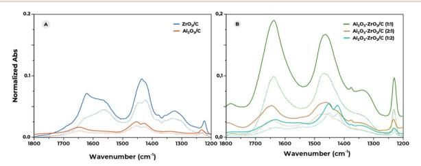
Fig. 4 IR spectra of CO<sub>2</sub> adsorption of pure oxides (A) and mixed oxides (B) with the solid lines corresponding to stabilization of 25 mbar CO<sub>2</sub> and dotted lines to CO<sub>2</sub> outgassing (5  $\times$  10<sup>-5</sup> mbar).
