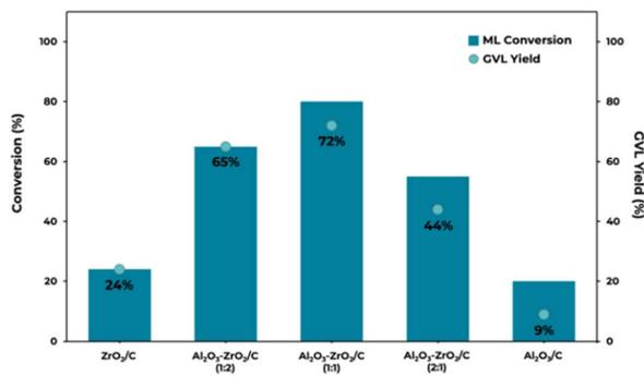
Fig. 6 Catalyst screening in the CTH of methyl levulinate into  $\gamma$ -valerolactone promoted by MOF-derived Al<sub>2</sub>O<sub>3</sub>-ZrO<sub>2</sub>/C catalysts by using 2-propanol as an H-source (reaction conditions: 0.5 mL min<sup>-1</sup> flow rate; ML 0.2 M in 2-propanol; 0.500 g of catalyst; 30 bar pressure; time on stream: 30 min; reaction temperature: 200 °C).
