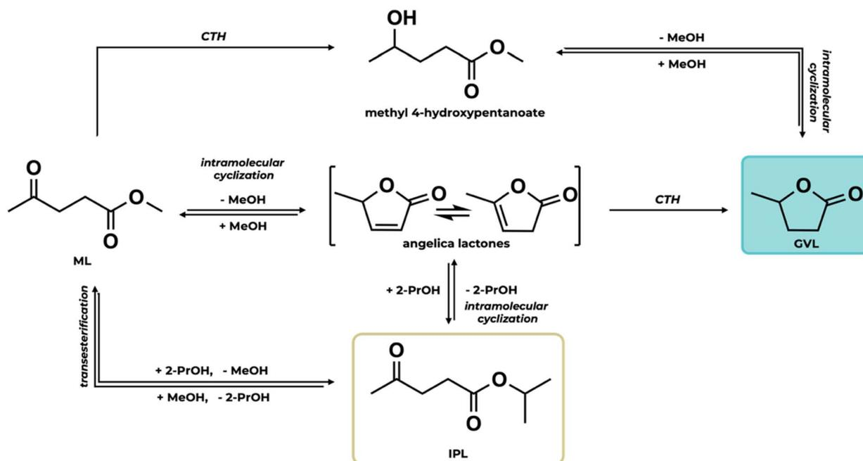
Scheme 2 Reaction pathways in the CTH of methyl levulinate (ML) with 2-propanol to GVL under continuous flow conditions.
