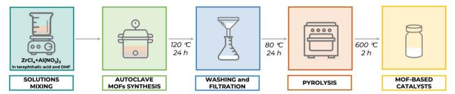
Scheme 1 Schematic representation of the synthesis and preparation process of the bimetallic MOF-derived Al<sub>2</sub>O<sub>3</sub>–ZrO<sub>2</sub>/C catalysts.
