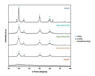
Fig. 1 XRD patterns of calcined MOF-derived Al<sub>2</sub>O<sub>3</sub>-ZrO<sub>2</sub>/C catalysts.
