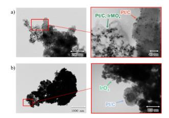
Fig. 6 TEM images of delaminated particles; (a) is a mixture of Pt/C and Pt/C, IrMO<sub>x</sub> sides from the fuel cell membrane, and (b) is a mixture of Pt/C and IrOx sides from water electrolyser membrane.
