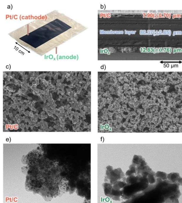
**Fig. 2** (a) Shows a photograph of the water electrolyser CCM. (b) Provides a SEM image of the water electrolyser CCM cross-section. (c) and (d) Illustrate the Pt/C and IrO<sub>x</sub> layers. (e) and (f) Present TEM images of the Pt/C and IrO<sub>x</sub> particles, respectively.
