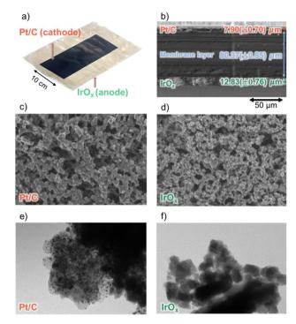
Fig. 2 (a) Shows a photograph of the water electrolyser CCM. (b) Provides a SEM image of the water electrolyser CCM cross-section. (c) and (d) Illustrate the Pt/C and IrO $_x$  layers. (e) and (f) Present TEM images of the Pt/C and IrO $_x$  particles, respectively.
