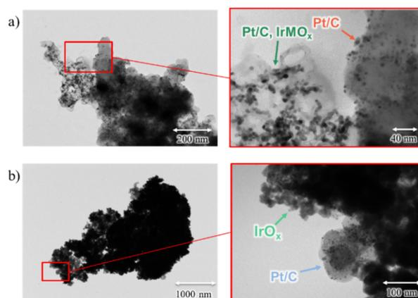
Fig. 6 TEM images of delaminated particles; (a) is a mixture of Pt/C and Pt/C, IrMO<sub>x</sub> sides from the fuel cell membrane, and (b) is a mixture of Pt/C and IrO<sub>x</sub> sides from water electrolyser membrane.
