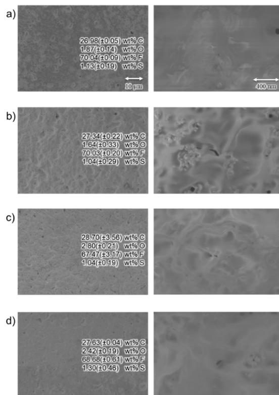
Fig. 5 SEM images of delaminated membranes; (a) and (b) are Pt/C and Pt/C, IrMO<sub>x</sub> sides of the fuel cell membrane, (c) and (d) are Pt–C and IrO<sub>x</sub> sides of water electrolyser membrane.
