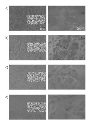
Fig. 5 SEM images of delaminated membranes; (a) and (b) are Pt/C and Pt/C, IrMO, sides of the fuel cell membrane, (c) and (d) are Pt-C and IrO<sub>v</sub> sides of water electrolyser membrane.
