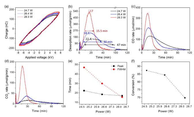
Fig. 5 Influence of plasma power on the reaction/desorption behaviors of  $CO_2$  captured by CaO. (a) Q-V Lissajous curve of the discharge; (b)–(d) desorption rates of  $CO + CO_2 + CH_4$ , CO, and  $CO_2$ , respectively, and (e) peak and FWHM times of the desorption rate, and (f)  $CO_2$  conversion as a function of power. Reaction conditions: 0.1 g of " $CaCO_3$ " (CaO after DAC for 24 h), 10%  $H_2/Ar$  30 mL min<sup>-1</sup>.
