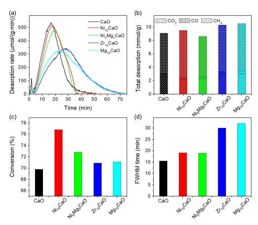
Fig. 3 Influence of second metal/metal oxide on the reaction/desorption behaviors. (a) Desorption rates of CO + CO<sub>2</sub> + CH<sub>4</sub>, (b) cumulative total desorption of CO + CO<sub>2</sub> + CH<sub>4</sub>, (c) CO<sub>2</sub> conversion, and (d) FWHM time. Reaction conditions:  $0.1 \, \text{g}$  of sample (after DAC for 24 h),  $10\% \, \text{H}_2/\text{Ar}$ 30 mL min<sup>-1</sup>, plasma power 28.3 W. More detailed results can be found in Fig. S7.†
