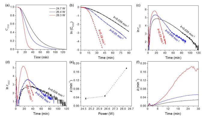
Fig. 6 Kinetic analysis of the data obtained at different plasma power. (a) Normalized  $CO_2$  concentration (remaining in the sorbent) as a function of time (calculated using eqn (12)) (b) normalized  $CO_2$  concentration modeled based on eqn (8)); (c) rate of  $CO_2$  desorption modeled based on eqn (10); (d) rate of  $CO_2$  desorption modeled based on eqn (9); (e) rate constant k as a function of plasma power; (f) changes in rate constant k before reaching a steady state.
