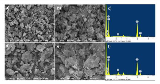
Fig. 3 (a and b) SEM images of [DEDSA][MnO<sub>4</sub>], (c) EDX analysis of [DEDSA][MnO<sub>4</sub>], (d and e) SEM images of [DSPZ][MnO<sub>4</sub>]<sub>2</sub>, and (f) EDX analysis of [DSPZ][MnO<sub>4</sub>]<sub>2</sub>.
