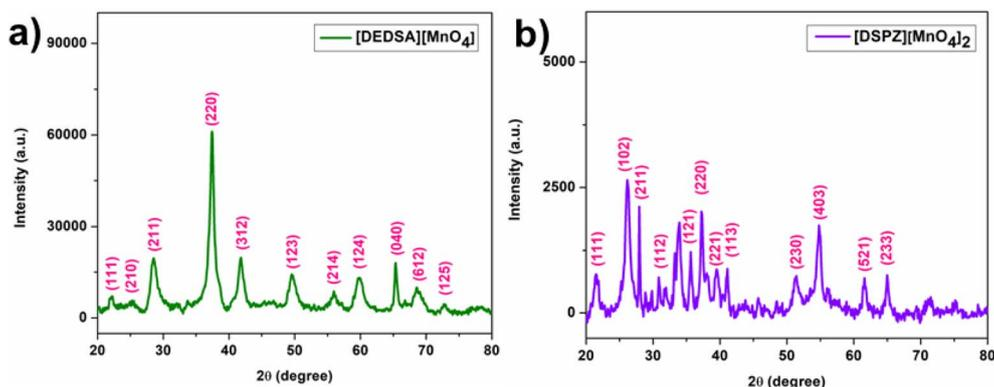
Fig. 4 PXRD patterns of (a) [DEDSA][MnO<sub>4</sub>] and (b) [DSPZ][MnO<sub>4</sub>]<sub>2</sub>.
