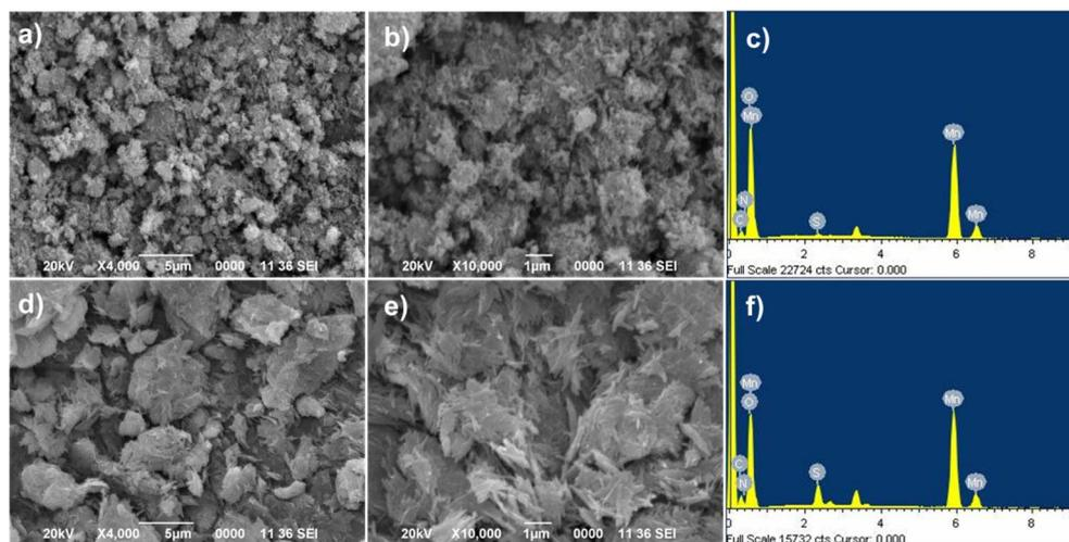
Fig. 3 (a and b) SEM images of [DEDSA][MnO<sub>4</sub>], (c) EDX analysis of [DEDSA][MnO<sub>4</sub>], (d and e) SEM images of [DSPZ][MnO<sub>4</sub>]<sub>2</sub>, and (f) EDX analysis of [DSPZ][MnO<sub>4</sub>]<sub>2</sub>.
