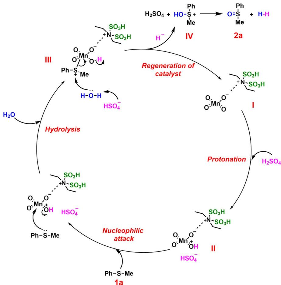
Scheme 3 A plausible mechanism for the oxidation of sulfides to sulfoxides with the [DEDSA][MnO<sub>4</sub>] salt.
