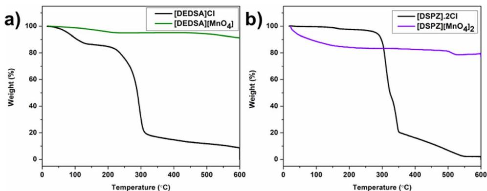
Fig. 2 Comparative thermogravimetric analysis curves of (a) [DEDSA]Cl and [DEDSA][MnO<sub>4</sub>]<sub>2</sub> and (b) [DSPZ]·2Cl and [DSPZ][MnO<sub>4</sub>]<sub>2</sub>.
