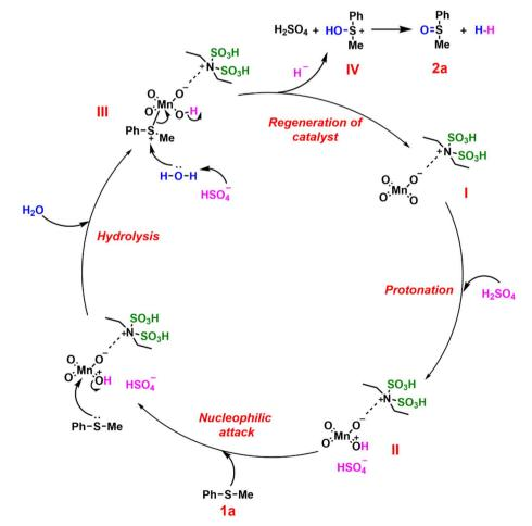
Scheme 3 A plausible mechanism for the oxidation of sulfides to sulfoxides with the [DEDSA][MnO<sub>4</sub>] salt.
