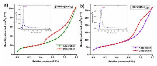
BET isotherms and BJH plots (insets) of (a) [DEDSA][MnO<sub>4</sub>] and (b) [DSPZ][MnO<sub>4</sub>]<sub>2</sub>.
