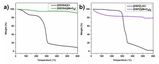
Comparative thermogravimetric analysis curves of (a) [DEDSA]Cl and [DEDSA][MnO<sub>4</sub>]<sub>2</sub> and (b) [DSPZ]·2Cl and [DSPZ][MnO<sub>4</sub>]<sub>2</sub>.
