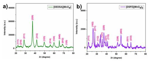
Fig. 4 PXRD patterns of (a) [DEDSA][MnO<sub>4</sub>] and (b) [DSPZ][MnO<sub>4</sub>]<sub>2</sub>
