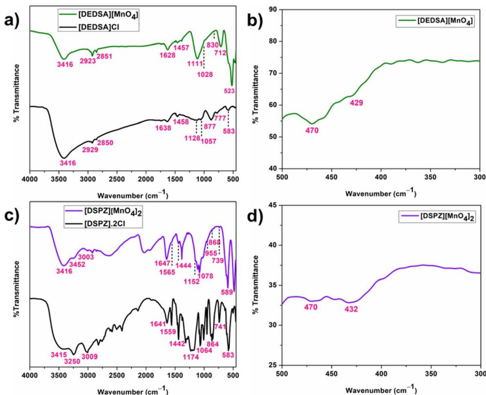
Fig. 1 Comparative FT-IR spectra of (a) [DEDSA]Cl and [DEDSA][MnO<sub>4</sub>], (b) far-IR analysis of [DEDSA][MnO<sub>4</sub>], (c) comparative FT-IR spectra of [DSPZ]·2Cl and [DSPZ][MnO<sub>4</sub>]<sub>2</sub>, and (d) far-IR analysis of [DSPZ][MnO<sub>4</sub>]<sub>2</sub>.
