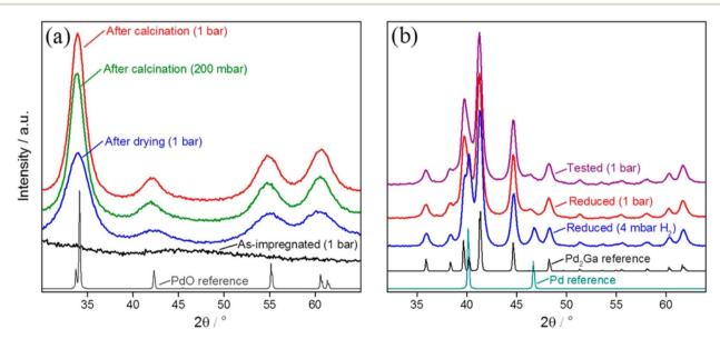
Fig. 12 (a) XRD patterns obtained from the impregnated, dried, and calcined catalyst precursor at room temperature and atmospheric pressure, and (b) from the reduced and tested GaPd<sub>2</sub>/SiO<sub>2</sub> catalyst for CO<sub>2</sub> hydrogenation. Reprinted with permission from ref. 333. Copyright 2015 American Chemical Society.
