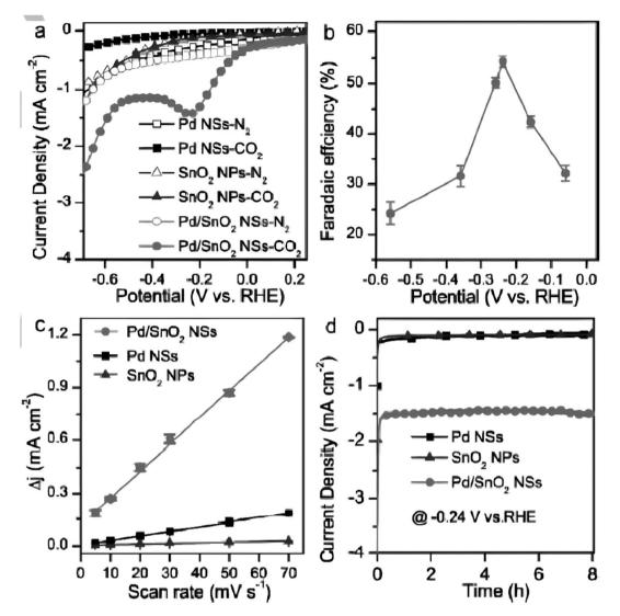
Fig. 14 Electrochemical characterization studies of  $Pd/SnO_2$  NSs (Pd:Sn=1:1) in comparison with Pd NSs and  $SnO_2$  NPs. (a) LSV curves obtained in 0.1 M NaHCO<sub>3</sub> solution. (b) FE for CH<sub>3</sub>OH at various applied potentials. (c) Charging current density differences plotted against scan rates. (d) Chronoamperometry studies of different catalysts. Reprinted with permission from ref. 390. Copyright permission from 2018 Wiley-VCH Verlag GmbH & Co. KGaA, Weinheim.
