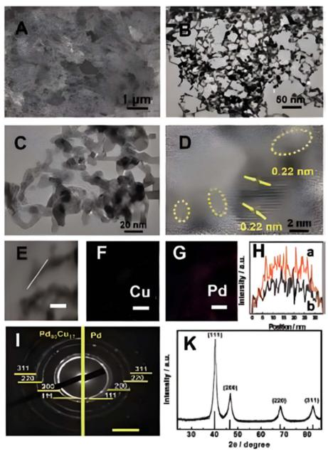
Fig. 15 (A) SEM, (B) and (C) TEM, (D) HR-TEM, and (E)–(G) EDX mapping images (scale bar: 20 nm). (H) Distribution of Pd (a) and Cu (b) in  $Pd_{83}Cu_{17}$  by line-scan analysis. (I) SAED pattern of the  $Pd_{83}Cu_{17}$  and pure Pd (scale bar: 10 1 nm@1). (K) XRD pattern of the  $Pd_{83}Cu_{17}$  aerogel. Reprinted with permission from ref. 389 Copyright permission from 2018 Wiley-VCH Verlag GmbH & Co. KGaA, Weinheim.
