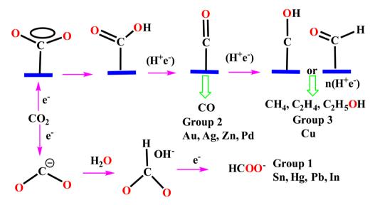
Fig. 5 Reaction mechanism of the electrochemical CO<sub>2</sub>RR on metal electrodes in aqueous solutions.<sup>224</sup>
