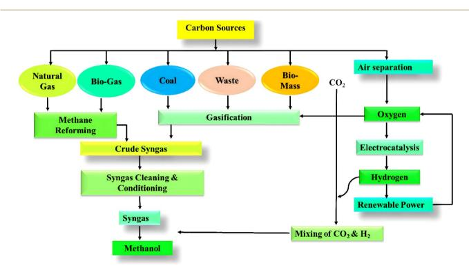
Fig. 1 Overview of key methanol synthesis methods using diverse carbon sources.
