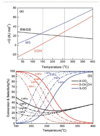
Fig. 3 (a) Free energy of methanol synthesis (MS) from  $CO_2$ , RWGS and syngas hydrogenation (COH). (b) Equilibrium conversion-selectivity values of the  $CO_2$ -hydrogenation reaction at various pressures Reprinted with permission from ref. 156. Copyright 2020 Royal Society of Chemistry.
