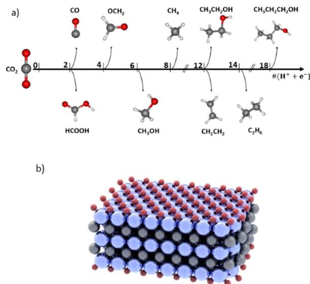
Fig. 1 (a) Products emerging from the electrochemical reduction of  $\text{CO}_2$  with multiple proton-coupled electron transfer (PCET) steps. (b) Schematic of an MXene support used in this study:  $\text{Ti}_3\text{C}_2\text{O}_2$ .
