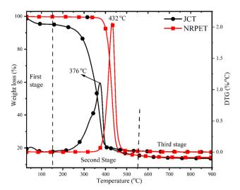
Fig. 4 Thermal stability analysis of JCT and NRPET at 10  $^{\circ}$ C min $^{-1}$
