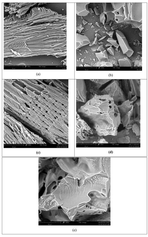
Fig. 9 SEM analysis of (a) JCTB, (b) NRPETB, (c) JCTB + NRPETB (30 wt%), (d) JCTB + NRPETB (50 wt%) and (e) JCTB + NRPETB (80 wt%).
