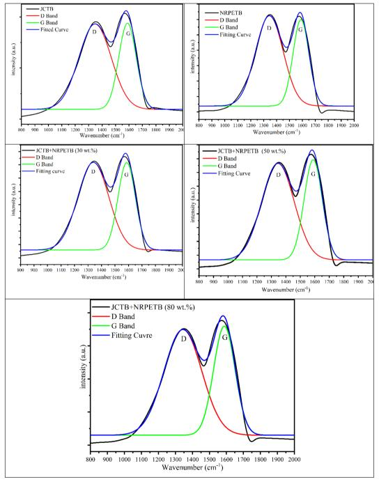
Fig. 8 Raman analysis of char derived at 500 °C.
