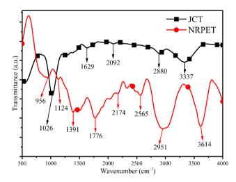
Fig. 5 FTIR analysis of JCT and NRPET.
