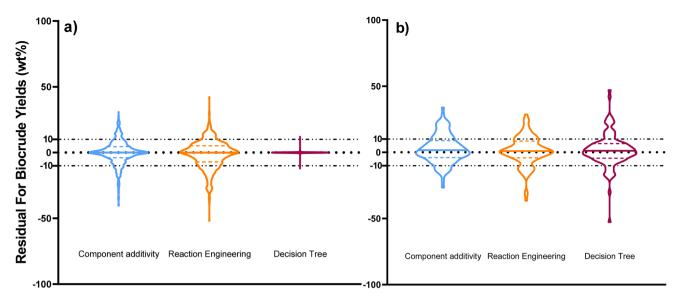
Residuals from calculating biocrude yields with each new model using a violin plot. The outer curve is the distribution of the residuals, the solid line in the middle is the median residual, and the dashed lines are the upper and lower quartiles: (a) Model fitting, (b) model predictions.
