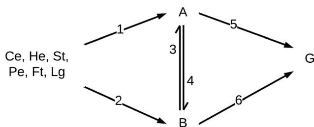
Fig. 3 Reaction network for modeling HTL of biomass.
