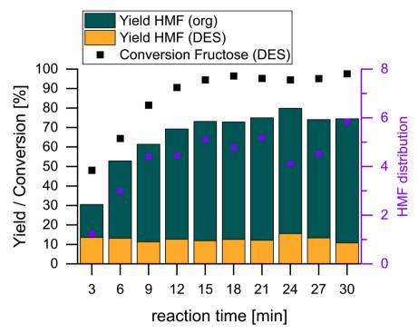
Fig. 4 Progress of the biphasic dehydration of Fru to HMF. Reaction conditions: 18 q ChCl, 4.5 q Fru, ChCl: Fru (5:1), V<sub>solvent</sub> = 150 mL, T = 80 °C, t=15 min,  $\omega=400$  rpm,  $c_{\mathrm{H_4SiW_{12}O_{40}}}=0.87$  mol $\%_{\mathrm{Fru}}$ .
