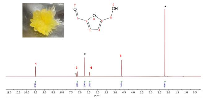
Recorded <sup>1</sup>H-NMR spectrum of an HMF crystal dissolved in CDCl<sub>3</sub> with mesitylene as a standard (400 MHz, \* = mesitylene, # = CDCl<sub>3</sub>).
