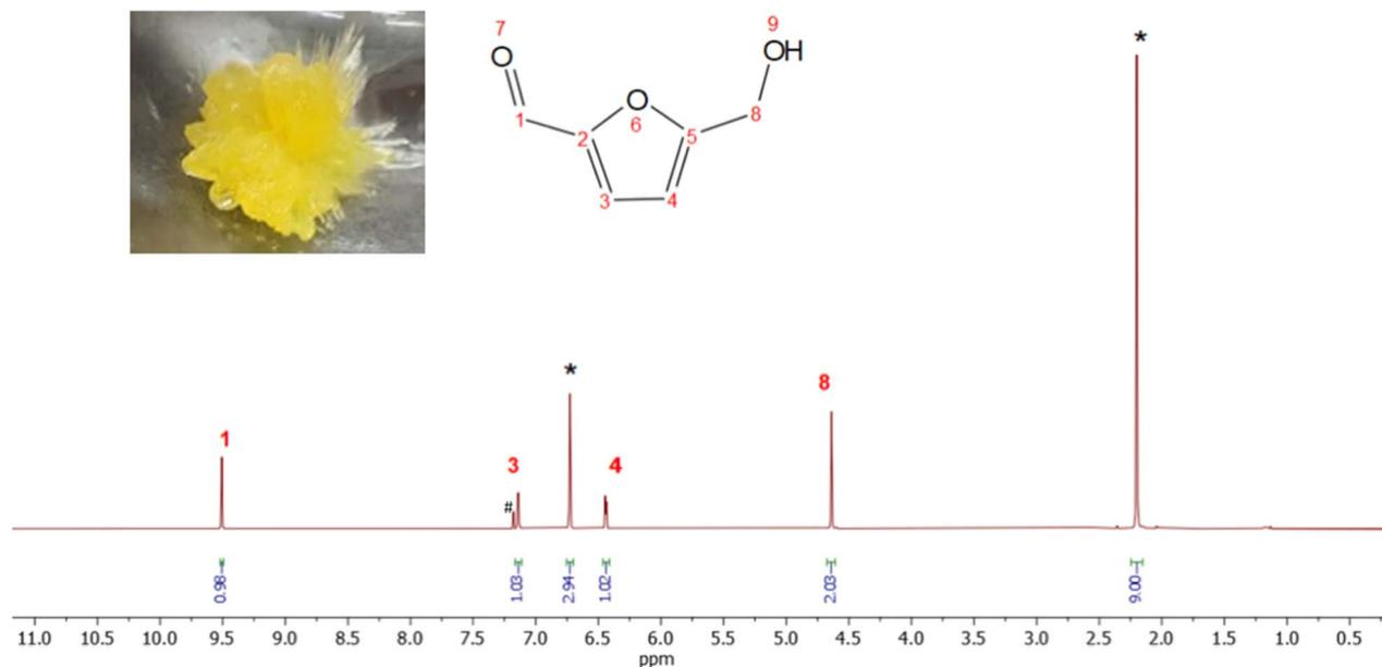
Fig. 7 Recorded  $^1\text{H}$ -NMR spectrum of an HMF crystal dissolved in  $\text{CDCl}_3$  with mesitylene as a standard (400 MHz, \* = mesitylene, # =  $\text{CDCl}_3$ ).
