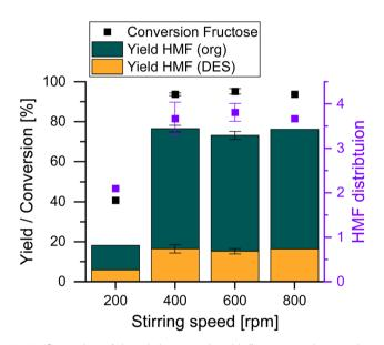
Fig. 3 Screening of the stirring speed and influence on the reaction. Reaction conditions: 18 g ChCl, 4.5 g Fru, ChCl: Fru (5:1),  $V_{\rm solvent}=150$  mL, T=80 °C, t=15 min,  $c_{\rm H_4SiW_{12}O_{40}}=0.87$  mol%<sub>Fru</sub>.
