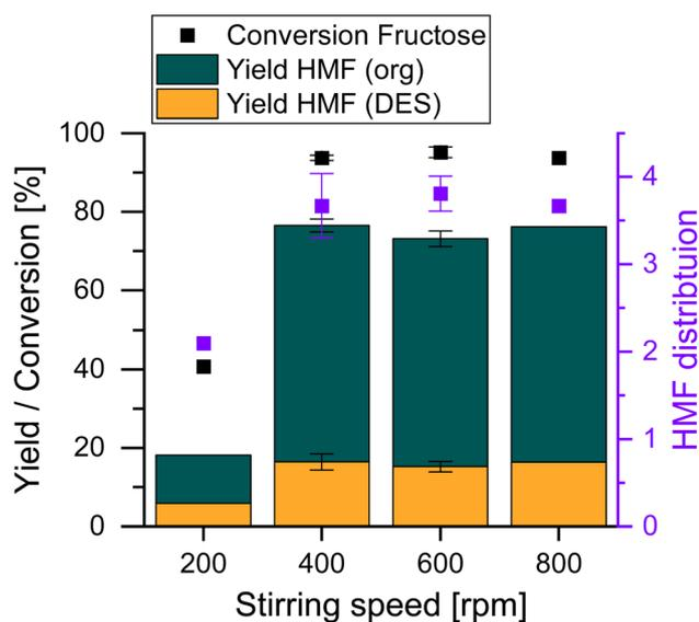
Fig. 3 Screening of the stirring speed and influence on the reaction. Reaction conditions: 18 g ChCl, 4.5 g Fru, ChCl : Fru (5 : 1),  $V_{\text{solvent}} = 150 \text{ mL}$ ,  $T = 80 \text{ }^\circ\text{C}$ ,  $t = 15 \text{ min}$ ,  $\text{C}_{\text{H}_4\text{SiW}_{12}\text{O}_{40}} = 0.87 \text{ mol}\%_{\text{Fru}}$ .
