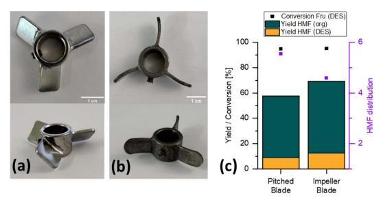
Fig. 2 Images of (a) the pitched blade and (b) the impeller blade used to mix the biphasic reaction system for the production of HMF. (c) Reaction performance and HMF distribution in both phases achieved with both types of impellers. Reaction conditions: 18 g ChCl, 4.5 g Fru, ChCl: Fru (5: 1),  $V_{\text{solvent}} = 150 \text{ mL}$ ,  $T = 80 ^{\circ}\text{C}$ , t = 15 min,  $\omega = 600 \text{ rpm}$ ,  $c_{\text{H}_{a}\text{SiW}_{12}\text{O}_{a0}} = 0.87 \text{ mol}\%_{\text{Fru}}$ .
