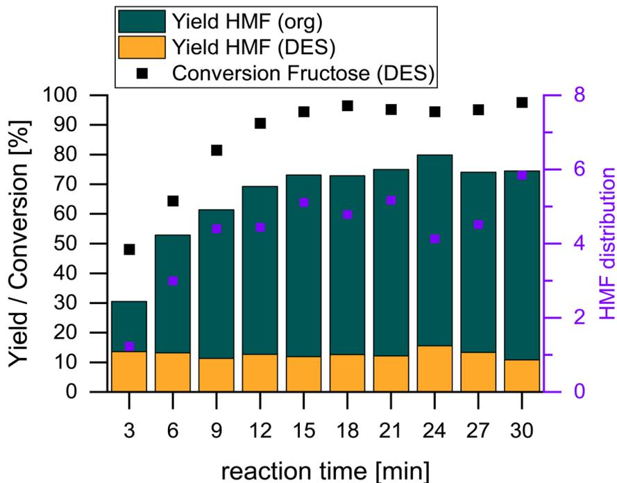
Fig. 4 Progress of the biphasic dehydration of Fru to HMF. Reaction conditions: 18 g ChCl, 4.5 g Fru, ChCl : Fru (5 : 1),  $V_{\text{solvent}} = 150$  mL,  $T = 80$  °C,  $t = 15$  min,  $\omega = 400$  rpm,  $C_{\text{H}_4\text{SiW}_{12}\text{O}_{40}} = 0.87$  mol% $_{\text{Fru}}$ .
