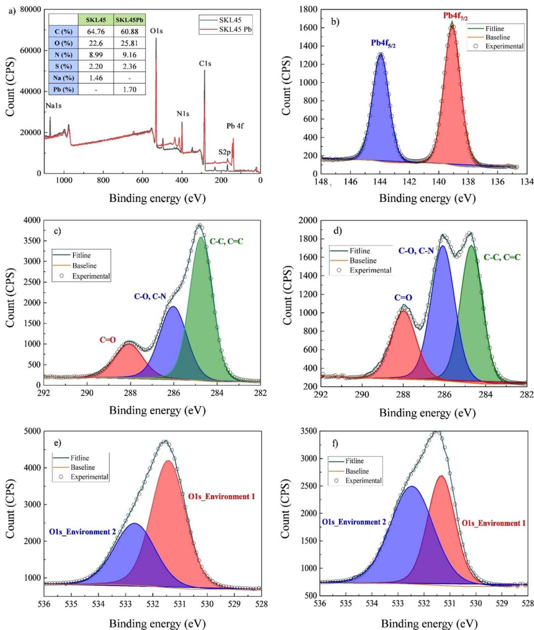
Fig. 5 XPS evaluation of the Pb(II) ion adsorption process on SKL45 including (a) survey spectra presenting the elemental composition; (b) wide scan region of the Pb<sub>4f</sub> for SKL45Pb; (c) wide scan region of the C 1s for SKL45; (d) wide scan region of the C 1s for SKL45Pb; (e) wide scan region of the O 1s for SKL45; and (f) wide scan region of the O 1s for SKL45 Pb.
