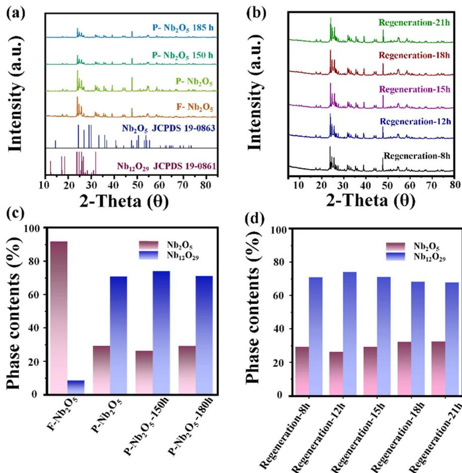
Fig. 3 X-ray diffraction (XRD) patterns and phase content of F-Nb<sub>2</sub>O<sub>5</sub>, P-Nb<sub>2</sub>O<sub>5</sub> and various catalysts to different reaction times (a and c); the XRD patterns and phase content of catalysts regenerated at 550 °C in an air atmosphere for varying durations (b and d).
