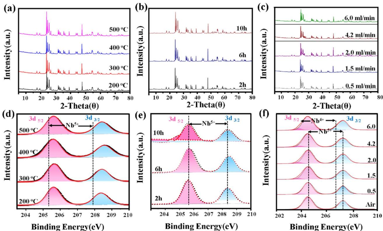
Fig. 7 Effect of temperature (a and d), time (b and e), and NH<sub>3</sub> (c and f) flow rate on the crystalline phases and oxidation states of niobium oxides: XRD and XPS.
