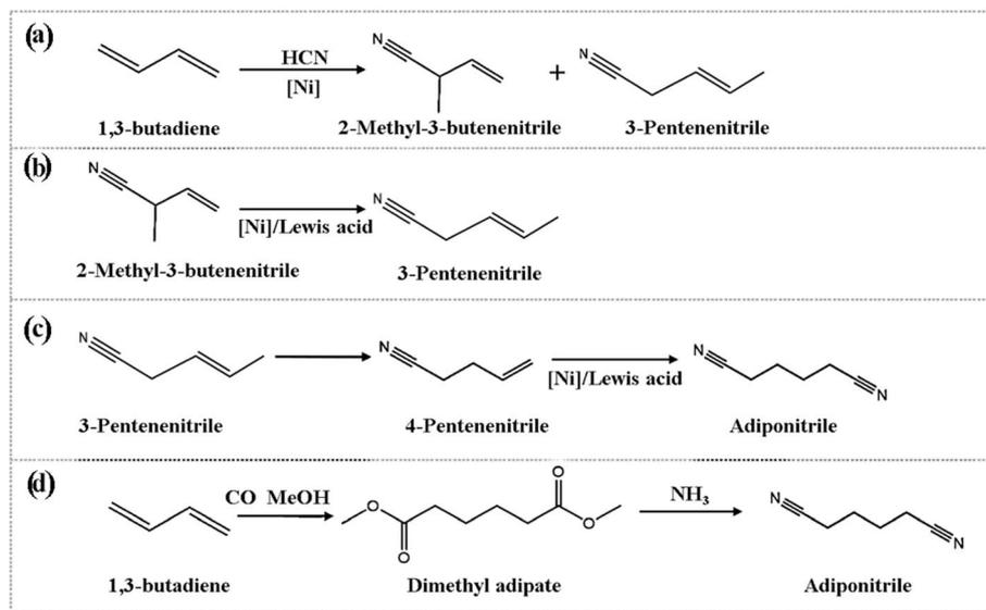
Fig. 1 Cyanidation of butadiene for preparation of adiponitrile.
