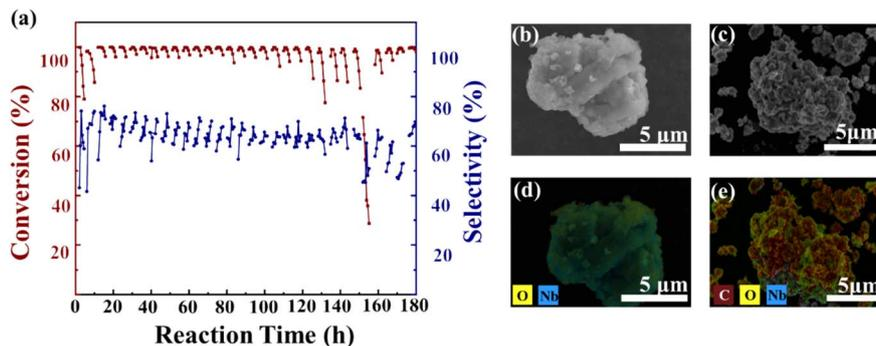
Fig. 2 (a) Catalyst reaction test ( $T = 375\text{ }^{\circ}\text{C}$ , DMA:  $18.3\text{ mmol h}^{-1}$ ,  $\text{NH}_3$ :  $4.9\text{ L h}^{-1}$ ,  $\text{NH}_3/\text{DMA}$  12 and LHSV  $2.4\text{ h}^{-1}$ ); SEM and EDS data of the catalyst before (b and d) and after the reaction (c and e).
