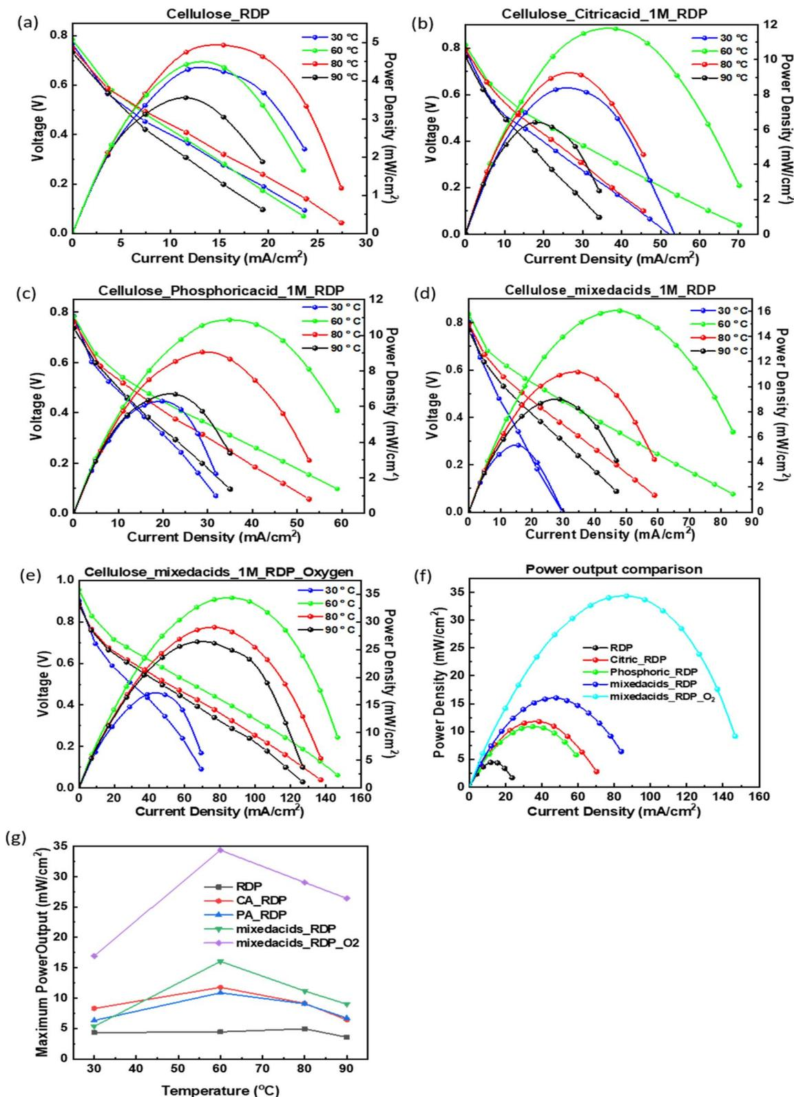
Fig. 2 Polarization curves for cellulose/RDP membrane with (a) no treatment (b) citric acid (c) phosphoric acid (d) mixed acids (e) mixed acids run in an oxygen environment (f) comparison of the max power performance for corresponding MEA (g) comparison of the power performance as a relation of temperature for each MEA.
