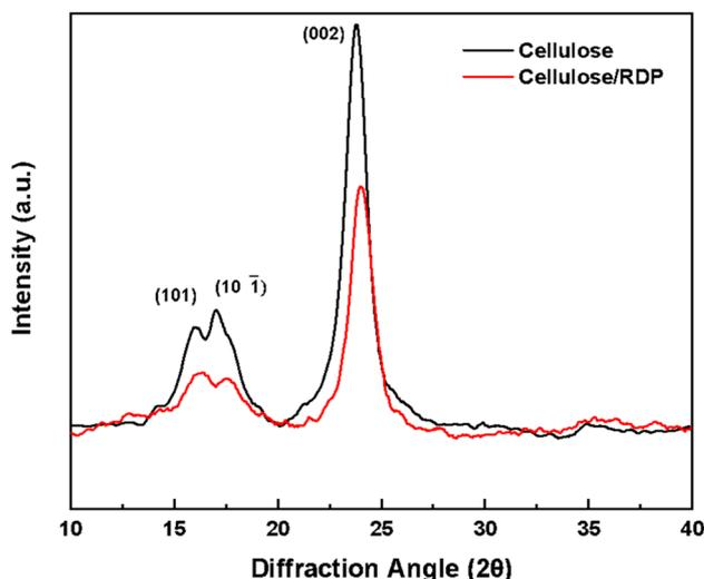
Fig. 5 XRD results of cellulose filter, cellulose/RDP membranes.
