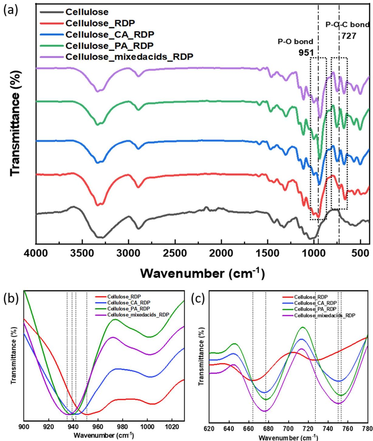
Fig. 6 (a) FTIR and (b and c) magnified dashed square region in (a) of the cellulose membrane, cellulose/RDP membrane and cellulose/RDP membrane treated with various acids.
