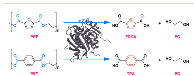
Scheme 1 Structure of PEF vs. PET and principle of enzymatic hydrolysis. The enzyme structure is ISPETase<sup>wt</sup> (PDB-ID: 6ILW).
