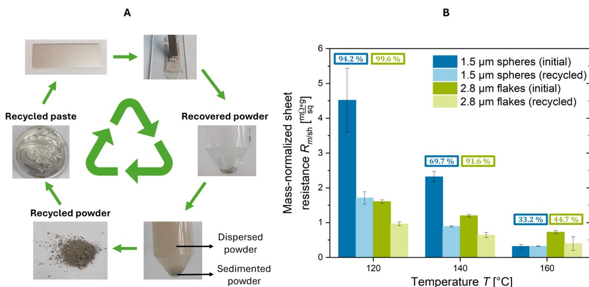
Fig. 3 The recycling of sintered prints of flakes and spheres followed the process shown in (A). Weight-normalized sheet resistances  $R_{m/sh}$  of prints of new ('initial') and recycled particles are shown in (B) as a function of sintering temperature  $T$  for 1.5  $\mu\text{m}$  spheres (blue) and 2.8  $\mu\text{m}$  flakes (green) treated for 30 min. The weight fractions indicate how much powder was recycled from the initial prints.
