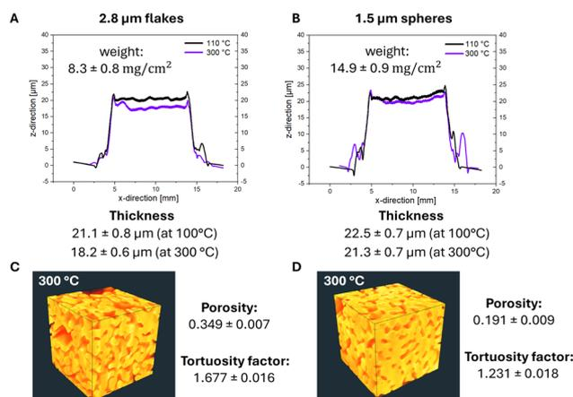
Fig. 2 Structures of sintered prints of flakes and spheres. Surface profiles of prints treated at 110 and 300 °C containing (A)  $2.8 \mu\text{m}$  flakes and (B)  $1.5 \mu\text{m}$  spheres from confocal microscopy. 3D reconstructions from FIB-SEM tomography of (C) prints based on  $2.8 \mu\text{m}$  flakes treated at 300 °C and (D) prints based on  $1.5 \mu\text{m}$  spheres treated at 300 °C.
