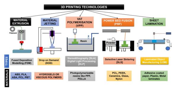
Fig. 2 Schematic illustration of various 3D printing processes for biodegradable material printing
