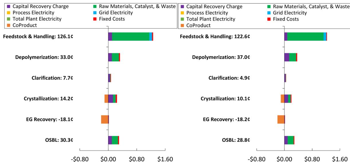
Fig. 5 Process contributors to the overall MSP of the PET enzymatic recycling processing at 50 kt year<sup>-1</sup> (left) and 100 kt year<sup>-1</sup> (right) of PET, respectively.
