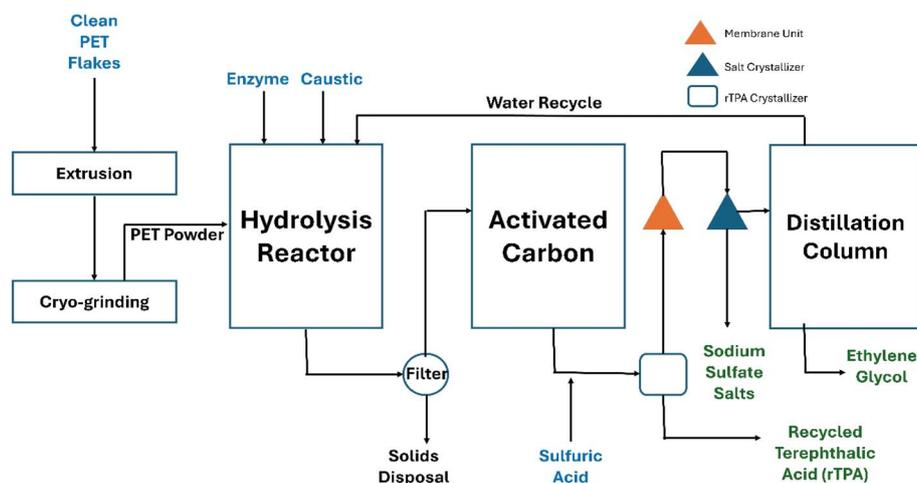
Fig. 1 Process flow diagram of enzymatic recycling of PET to rTPA and EG [adapted from Singh *et al.* (2021).<sup>25</sup>
