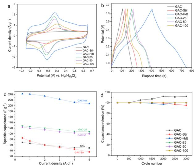
Fig. 6 Electrochemical performance performed in a three-electrode system: (a) CV curves at a scan rate of  $5 \text{ mV s}^{-1}$ ; (b) GCD curves at a current density of  $0.5 \text{ A g}^{-1}$ ; (c) specific capacitance at various current densities; (d) capacitance retention for 3000 cycles of GACs.
