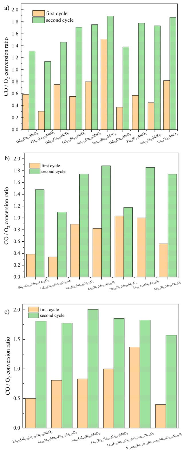
Fig. 9 CO/O<sub>2</sub> conversion ratios of (a) single doping, (b) double doping, and (c) multi doping of perovskites during two consecutive thermochemical cycles.
