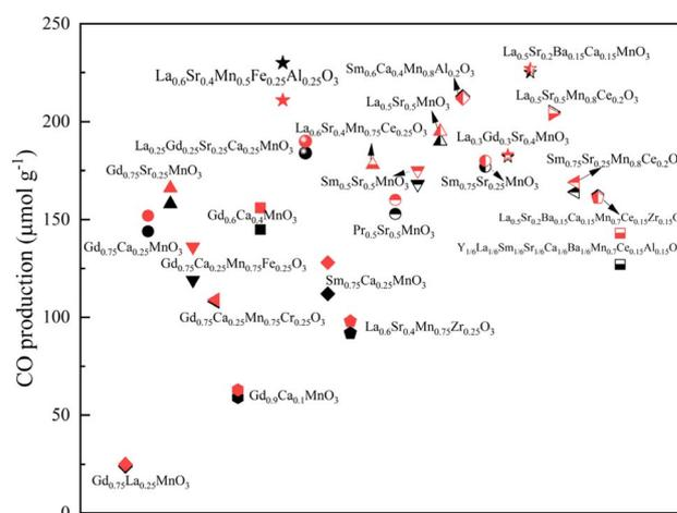
Fig. 8 CO production yields of 23 single, double, and multiple cation doped perovskites (black symbols represent the results of the first cycle and red symbols represent the results of the second cycle).
