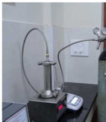
Fig. 2 Nanofiltration experimental set-up.
