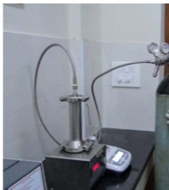
Fig. 2 Nanofiltration experimental set-up.
