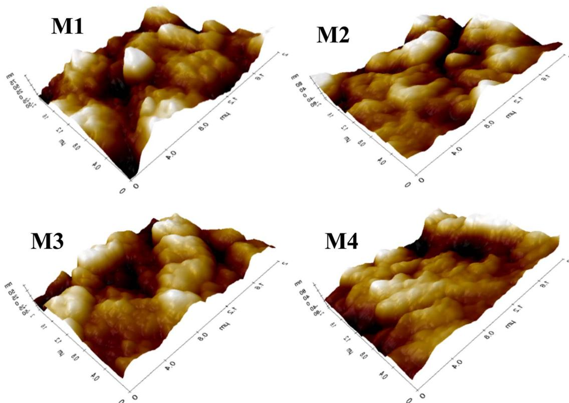
Fig. 6 Surface topology of the fabricated membranes.
