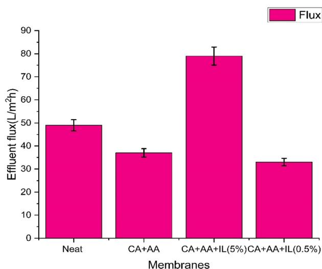
Fig. 12 Nanofiltration performance of industrial wastewater.
