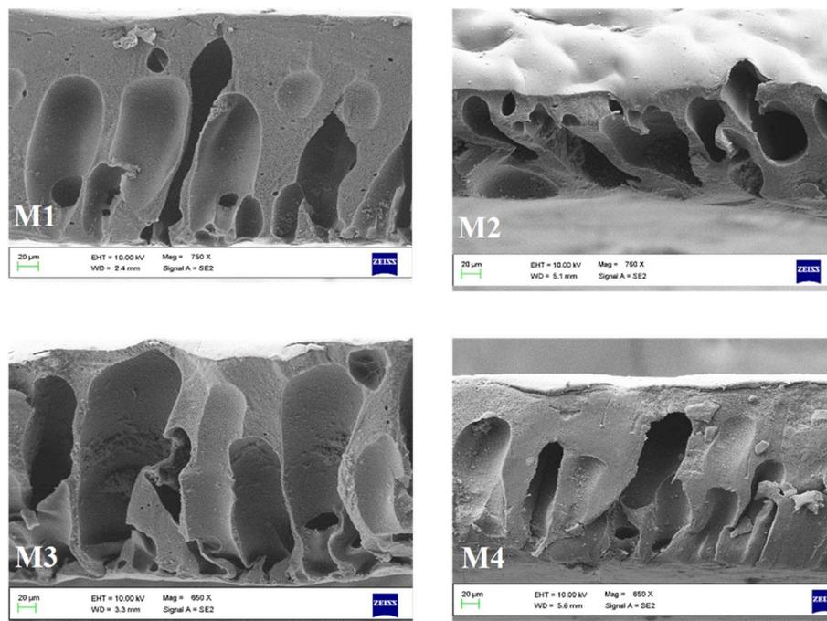
Fig. 5 Cross-sectional morphology of the fabricated membranes.
