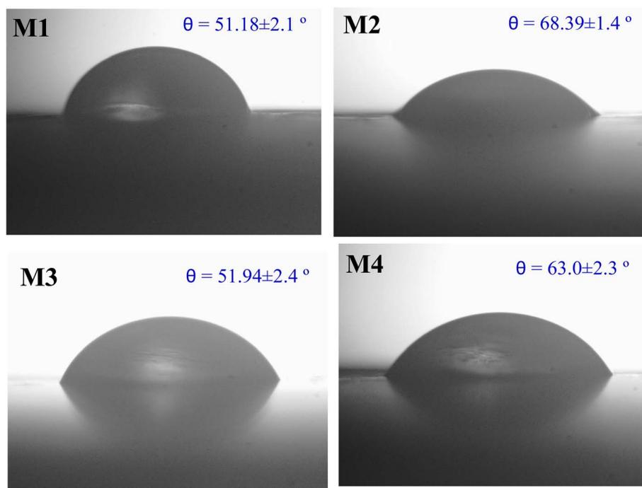
Fig. 7 Contact angle images of the fabricated membranes.
