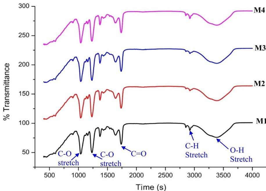
Fig. 3 FTIR spectra of the fabricated membranes.
