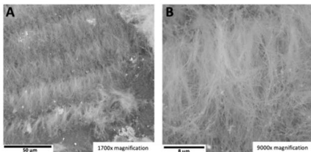
Fig. 4 DAC Genesis CNT products formed at  $\text{CO}_2$  sufficient conditions. 750 °C  $\text{Li}_2\text{CO}_3$  electrolyte electrolysis with a brass cathode and a stainless steel anode and case. SEM of the washed products: CNTs (A & B) 1700× and 9000× magnification.
