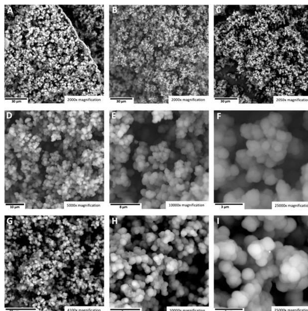
Fig. 5 DAC Genesis CNO products formed at  $\text{CO}_2$  insufficient conditions. 750 °C  $\text{Li}_2\text{CO}_3$  electrolyte electrolysis with a brass cathode and a stainless steel anode and case. SEM of the washed products: CNOs sample 1 (A–F) magnification at 2000×, 2000×, 2050×, 5000×, 10000×, 25000×. CNOs sample 2 (G–I) 4100×, 10000, and 25000×.
