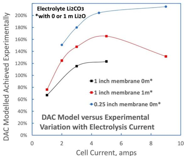
Fig. 3 A comparison of the DAC modelled  $\text{CO}_2$  diffusion limited currents and the experimentally measured DAC currents. Black data is measured with eqn (9) required airflow, and red and blue data with 2× higher flow.
