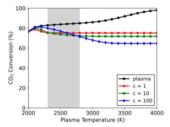
Fig. 6 CO<sub>2</sub> conversion in the plasma and in the afterglow (for three different c-factors: 1, 10 and 100) as a function of the plasma temperature, for the CO<sub>2</sub>/CH<sub>4</sub> ratio of 70/30. The range of plasma temperatures where the transition between the two afterglow effects occurs is indicated with a grey rectangle.
