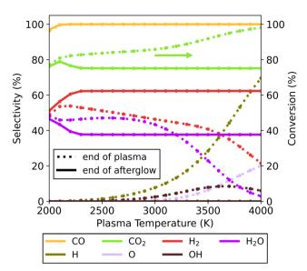
Fig. 4 Selectivity of the main species (above 5%) as a function of the plasma temperature, for the  $30/70 \, \text{CO}_2/\text{CH}_4$  ratio and c-factor of 1 (no enhance cooling), at the end of the plasma zone (point A in Fig. 1; dotted lines) and end of the afterglow (point B in Fig. 1; solid lines). Full conversion of  $\text{CH}_4$  is observed under all conditions, but not for  $\text{CO}_2$ , and therefore the  $\text{CO}_2$  conversion is also plotted (right y-axis).
