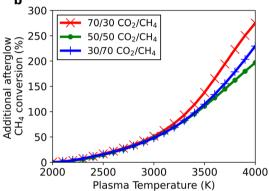
Fig. 7 Additional CO<sub>2</sub> (a) and CH<sub>4</sub> (b) conversion obtained in the afterglow relative to the conversion obtained in the plasma, as a function of plasma temperature, for three different CO<sub>2</sub>/CH<sub>4</sub> ratios (70/30, 50/50, 30/70) at  $\tau_{mix} = 10$  ms.
