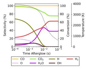
Fig. 5 Evolution of the selectivity of the main species in the afterglow, starting from a plasma temperature of 4000 K for the  $70/30 \text{ CO}_2/\text{CH}_4$  ratio and c-factor of 1. The evolution of the  $\text{CO}_2$  conversion and of the gas temperature (dotted line) are also plotted, and shown on the right axis
