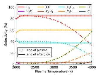
Fig. 3 Selectivity of the main species (above 5%) as a function of the plasma temperature, for the  $30/70 \text{ CO}_2/\text{CH}_4$  ratio and c-factor of 1 (no enhanced cooling), at the end of the plasma zone (point A in Fig. 1; dotted lines) and end of the afterglow (point B in Fig. 1; solid lines). Full conversion of CO<sub>2</sub> and CH<sub>4</sub> is observed under all conditions (except for 2000 K, as explained in the text).
