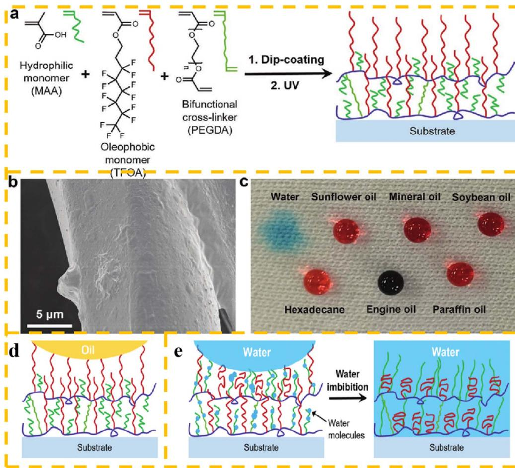
**Fig. 11** (a) Schematic of the formation of oleophobic and hydrophilic coating, (b) SEM image of the coated polyester fiber, and (c) photographs of water and oil drops on the coated polyester fabric. Water and clear oils were colored with methylene blue and oil red, respectively, for easy observation. (d) Repellency of fluorinated chains to oil and (e) the hydration of water molecules into the hydrophilic subsurface, as well as the subsequent water imbibition.
