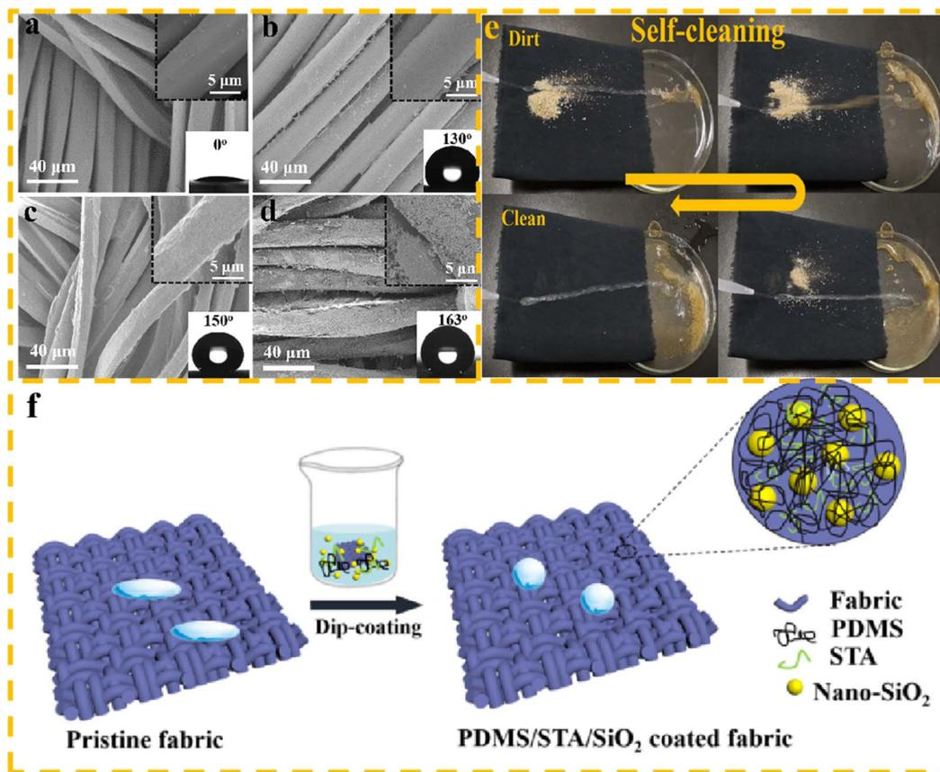
Fig. 4 Scanning electron microscopy (SEM) images of the fabrics: (a) pristine fabric, (b) PDMS-coated fabric, (c) PDMS/STA-coated fabric, and (d) PDMS/STA/SiO<sub>2</sub>-coated fabric. Insets show differently magnified SEM images and WCAs of the corresponding fabrics. (e) Self-cleaning property of the PDMS/STA/SiO<sub>2</sub>-coated fabric and (f) fabrication scheme for the preparation of the superhydrophobic coating on the fabric.
