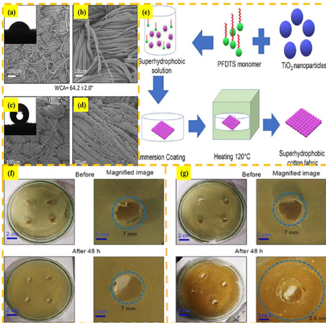
Fig. 5 SEM images of (a and b) coated and (c and d) uncoated cotton fabric with static contact angles of water, (e) schematic of the preparation of superhydrophobic cotton fabric using PFDTs and  $\text{TiO}_2$  nanoparticles in toluene, and (f and g) optical images of uncoated and coated cotton fabric before and after 48 h incubation with *E. coli* bacteria at  $37^\circ\text{C}$ , respectively. The inhibition zone (no growth of bacteria) near the coated fabric shows its antibacterial property.
