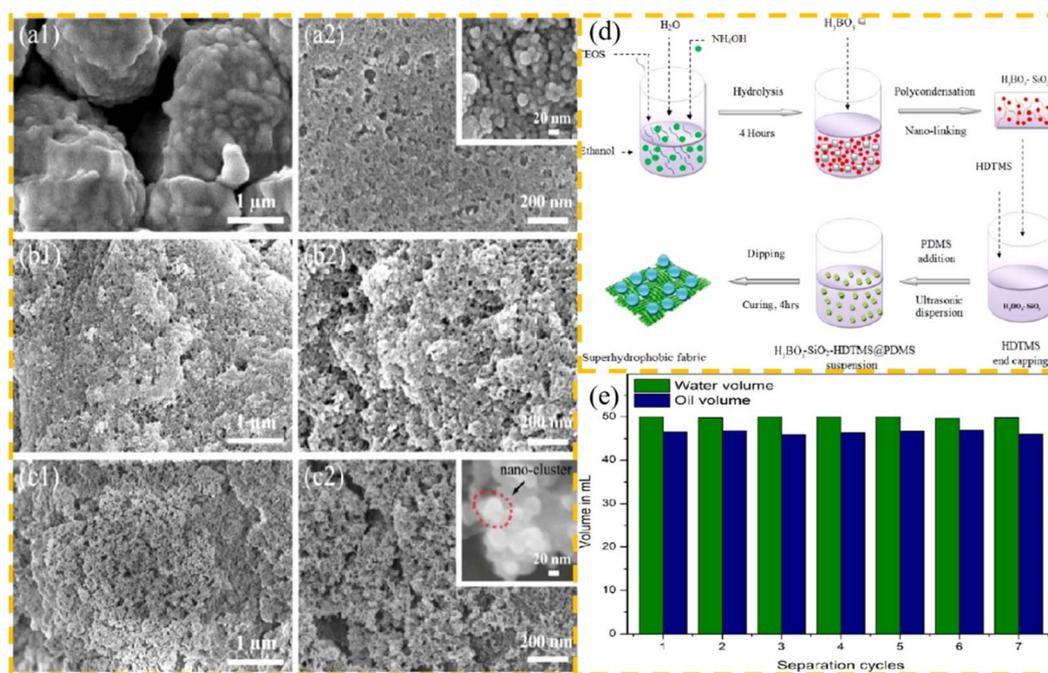
Fig. 6 SEM images of the coated fabric surface under different magnifications. Surface containing 21 wt% of SiO<sub>2</sub> (a1 and a2), 9 wt% of H<sub>3</sub>BO<sub>3</sub>-SiO<sub>2</sub> (b1 and b2), and 18 wt% of H<sub>3</sub>BO<sub>3</sub>-SiO<sub>2</sub> (c1 and c2), (d) modification process of fluorine-free superhydrophobic cotton fabric, and (e) oil/water volume (mL) after seven separation cycles by the coated superhydrophobic fabric.
