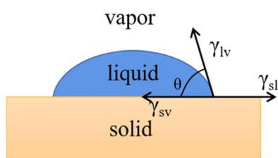
Fig. 2 Contact angle measured on a solid surface.
