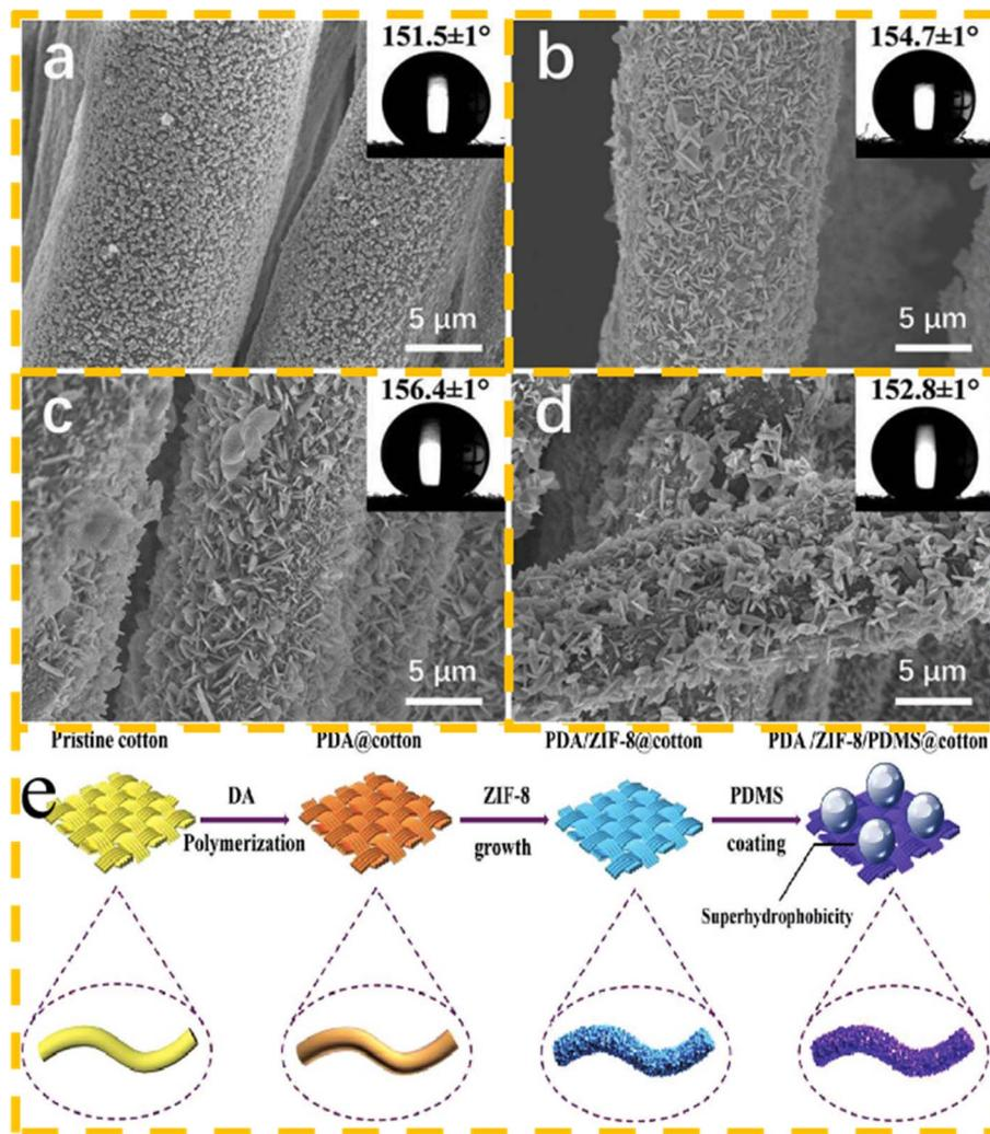
Fig. 10 SEM images (inset on the top right is the static behavior of the water droplet on the fabric) of PDA/ZIF-8/PDMS@ cotton fabric with (a)  $n(\text{Zn}^{2+}) : n(\text{Hmim}) = 1 : 16$ , (b)  $n(\text{Zn}^{2+}) : n(\text{Hmim}) = 1 : 10$ , (c)  $n(\text{Zn}^{2+}) : n(\text{Hmim}) = 1 : 8$ , (d)  $n(\text{Zn}^{2+}) : n(\text{Hmim}) = 1 : 6$ , and (e) schematic of the preparation of superhydrophobic PDA/ZIF-8/PDMS@ cotton fabric.
