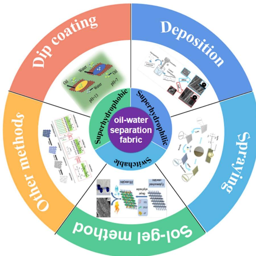
Fig. 1 Schematic of the methods for the fabrication of oil/water separation cotton fabrics, such as dip coating,<sup>60</sup> deposition,<sup>84</sup> spraying,<sup>88</sup> sol-gel method,<sup>132</sup> and other methods.<sup>103</sup>
