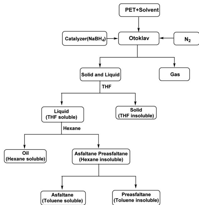
Fig. 16 Flow chart of the pyrolysis experiments. Reproduced with permission.<sup>123</sup> Copyright 2019, *IOP Conference Series: Earth and Environmental Science*.
