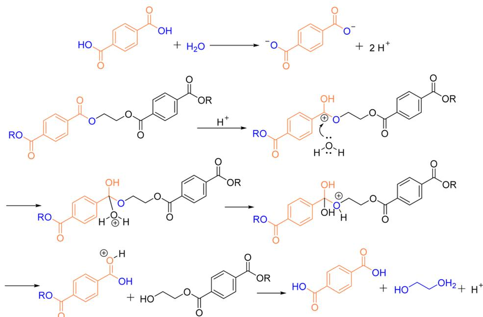
Fig. 11 PET hydrolysis mechanism with TPA as an acid catalyst. Reproduced with permission.<sup>99</sup> Copyright 2021, Elsevier Ltd.
