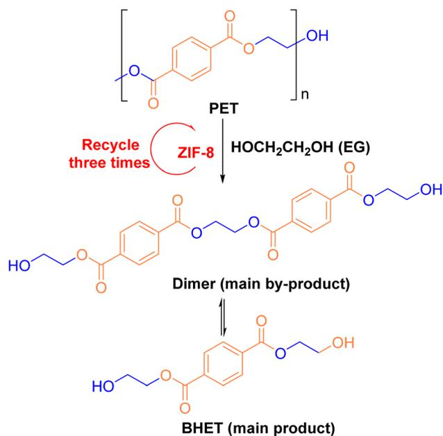
Fig. 7 ZIF-8 catalyzes the depolymerization process of PET. Reproduced with permission.<sup>63</sup> Copyright 2016, Springer Science, Business Media New York.
