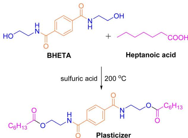
Fig. 14 Synthesis of plasticizer from bis(2-hydroxyethyl)terephthalamide (BHETA). Reproduced with permission.<sup>112</sup> Copyright 2013, Iran Polymer and Petrochemical Institute.
