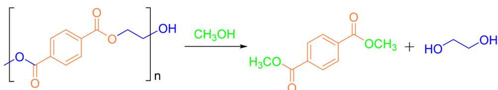
Fig. 3 The reaction formula of methanol alcoholsysis.
