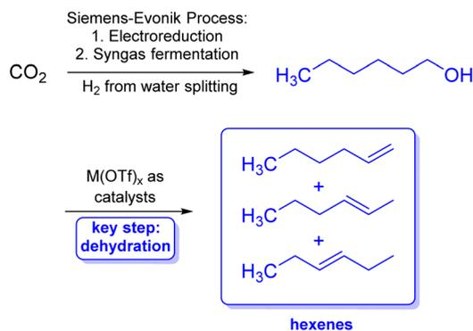
**Scheme 1** Overall process concept for producing hexenes from  $\text{CO}_2$ , water and renewable energy such as sunlight and wind in a chemo-enzymatic cascade with metal triflate dehydration as a key step.
