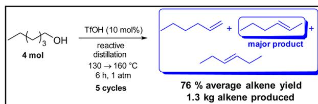
Scheme 6 100-fold scale up of the dehydration of 1-hexanol using TfOH for 5 cycles in batch. Reaction temperatures of the oil bath were  $150 \rightarrow 180^\circ\text{C}$  while inside temperatures were  $130\text{--}160^\circ\text{C}$ .
