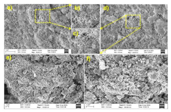
Fig. 3 (a and d) SEM images of NFNR; (b and c) zoom image of (a and d), and (e and f) SEM images of NFNR/rGO.
