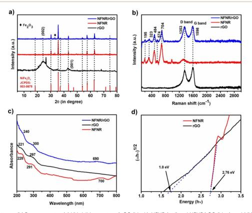
Fig. 1 (a) PXRD patterns, (b) Raman spectra, (c) UV visible spectra of rGO (black), NFNR (red) and NFNR/rGO (blue), and (d) Tauc plot of NFNR (red) and rGO (black).
