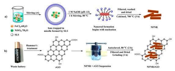
Scheme 1 Synthesis of (a) NFNR and (b) NFNR/rGO composites.
