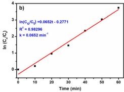
Fig. 8 (a) UV absorption spectra and (b)  $\ln(C_o/C_t)$  vs. time graph for BH degradation with NFNR/rGO under optimized conditions (12 mg catalyst, 60 min of irradiation time and pH = 2).
