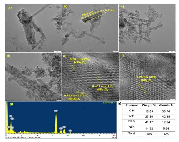
Fig. 4 TEM image of (a and b) NFNR, (c and d) NFNR/rGO showing the nanorod structure distributed on the rGO surface, (e and f) fringe pattern of NFNR/rGO obtained from HRTEM analysis, (g) EDX spectra and (h) average elemental distribution in the NFNR/rGO material.
