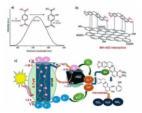
Fig. 11 (a) PL spectra indicated the formation of hydroxyl terephthalic acid (HTA), (b) BH-rGO  $\pi$ - $\pi$  interactions and (c) plausible mechanism for the photocatalytic degradation of BH on the NFNR/rGO surface under UV light irradiation.
