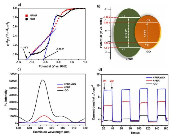
(a) Mott-Schottky plot for the flat band potential ( $V_{fb}$ ) of the NFNR (red line) and rGO (back line), (b) band edge structure showing the CB and VB potential of the NFNR and rGO, (c) PL spectra and (d) photocurrent responses of rGO (black line), NFNR (red line) and NFNR/rGO (blue line).
