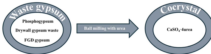
Fig. 5 The process of using industrial by-product waste to produce \text{CaSO}_4 \cdot 4\text{urea} . 38,40
