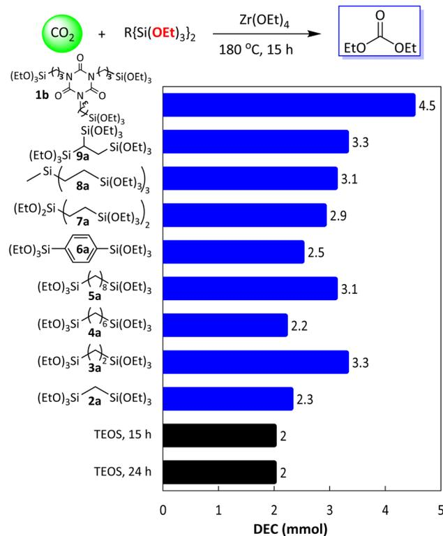
Fig. 6 Substrate scope. Reaction conditions: Si amount = 7.8 mmol,  $\text{Zr}(\text{OEt})_4 = 0.3$  g ( $\text{Si}/\text{Zr} = 7$ );  $\text{CO}_2$ , 5 MPa at room temperature. Yield was determined by GC or  $^1\text{H}$  NMR analysis using mesitylene as an internal standard.
