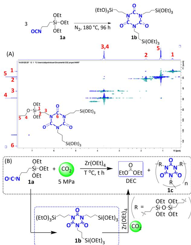
Fig. 4 (A) 2D (HSQC) NMR result of isocyanurate **1b**; (B) reaction pathway of DEC formation from CO<sub>2</sub> and **1a** through **1b** intermediate product. Reaction conditions: **1a**, 10 mL; N<sub>2</sub>, atmosphere; 180 °C; 96 h. Yield was determined by <sup>1</sup>H NMR spectroscopy.
