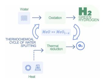
Hydrogen production through thermochemical processes
