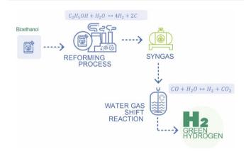
Wet ethanol reforming for hydrogen production.
