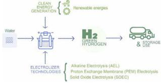
Green hydrogen production through water electrolysis.
