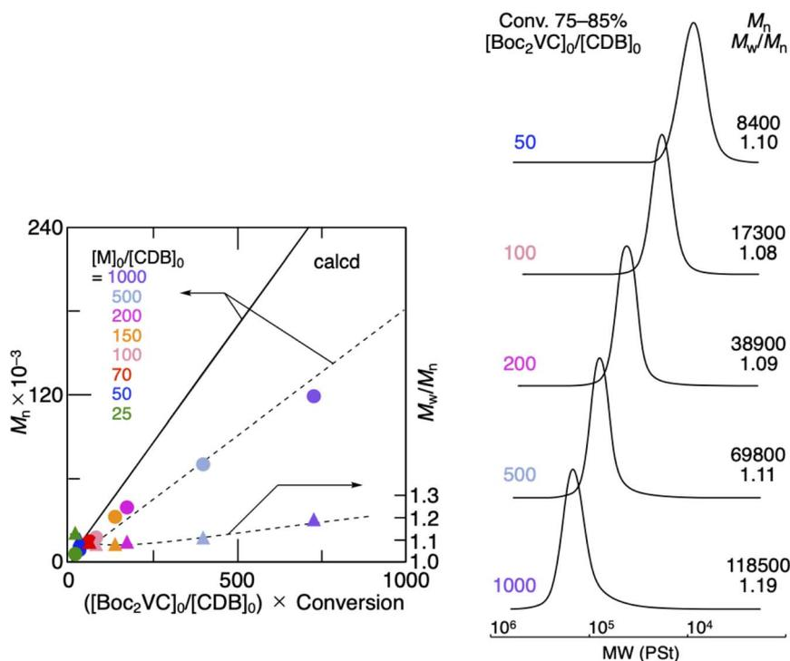
Fig. 2 SEC analysis of P(Boc<sub>2</sub>VC) obtained by RAFT polymerization of Boc<sub>2</sub>VC with varying feed ratios: [Boc<sub>2</sub>VC]<sub>0</sub>/[CDB]<sub>0</sub>/[AIBN]<sub>0</sub> = 2000/2.0/0.50, 2000/4.0/1.0, 2000/10/2.5, 1800/12/3.0, 2000/20/5.0, 1400/20/5.0, 1500/30/7.5, 1000/40/10 mM in ethyl acetate at 60 °C.
