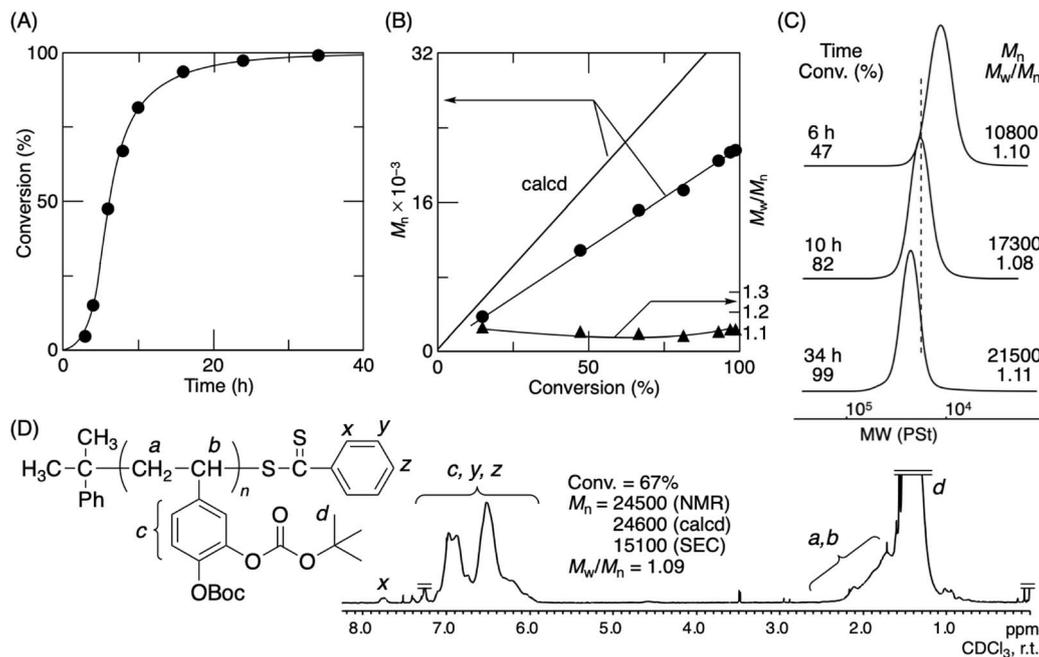
Fig. 1 Time-conversion (A),  $M_n$ (SEC) and  $M_w/M_n$  as a function of conversion (B), SEC curves (C), and <sup>1</sup>H NMR spectrum of the purified P(Boc<sub>2</sub>VC) (D) for RAFT polymerization of Boc<sub>2</sub>VC: [Boc<sub>2</sub>VC]<sub>0</sub>/[CDB]<sub>0</sub>/[AIBN]<sub>0</sub> = 2000/20/5.0 mM in ethyl acetate at 60 °C.
