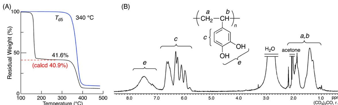
Fig. 3 TGA curves of P(Boc<sub>2</sub>VC) (black line) and P(Boc<sub>2</sub>VC) which had been heated at 200 °C for 15 min under N<sub>2</sub> (blue line) (A) and <sup>1</sup>H NMR spectra of the polymer deprotected by heat without any purification (B).
