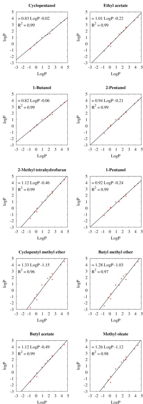
Fig. 3 Correlation between the  $\log P$  values of the employed biobased solvents and the experimental  $\log P$  in 1-octanol ( $\log P$ ). For each solvent, the linear regression equation is shown in addition to the coefficient of determination ( $R^2$ ).
