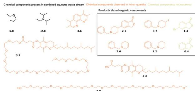
Fig. 5 Components of the aqueous medium from the extractions and their distribution coefficients between water and 1-octanol at pH 7.4,  $\log D$  (pH 7.4), from the chemical data sheets. Organic components with elevated concentrations in solution are highlighted in red, while compounds that are present in minor quantities are shown in orange. The highest concentrations are observed for 2-methyl tetrahydrofuran and *N,N*-diisopropylethylamine (upper left corner).
