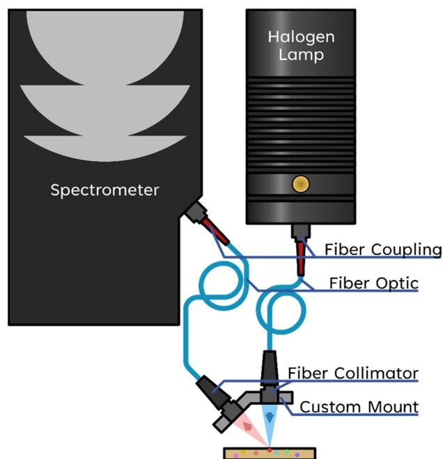
Fig. 1 Schematic of the near infrared (NIR) instrument. A broadband light source is focused onto a sample and the remitted light is collected at a  $45^\circ$  angle between the illumination and collection sources. The collected light is sent to a spectrometer for measurement, as described in the text.
