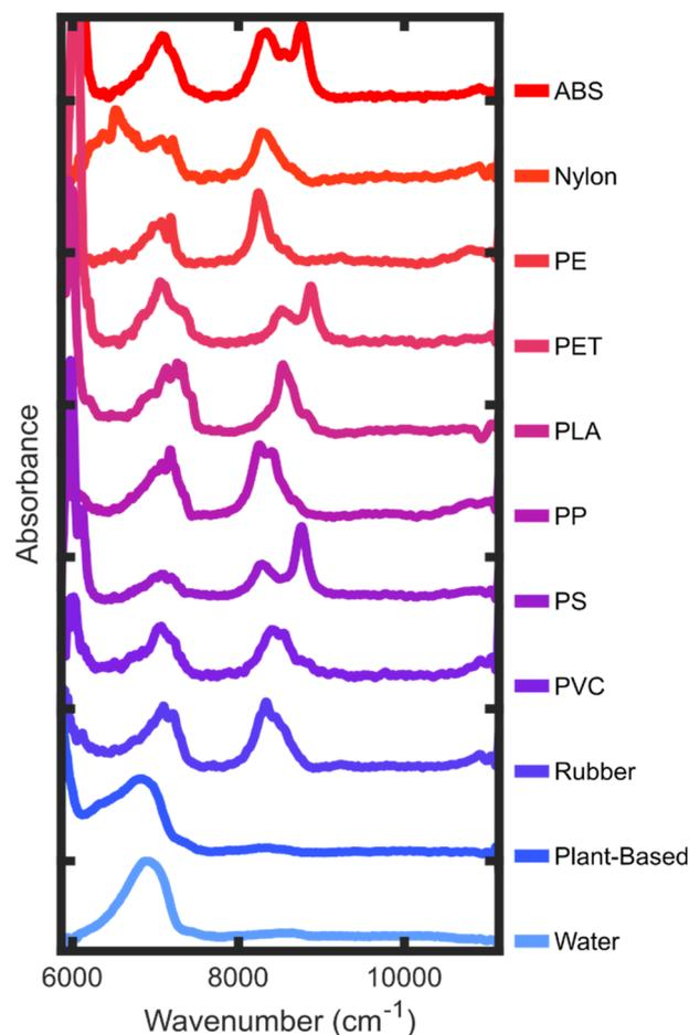
Fig. 4 Averaged absorbance spectra of each category of material. Frequency in  $\text{cm}^{-1}$  is on the x-axis and absorbance is on the y-axis. The definition of each plastic is included in the Methods.
