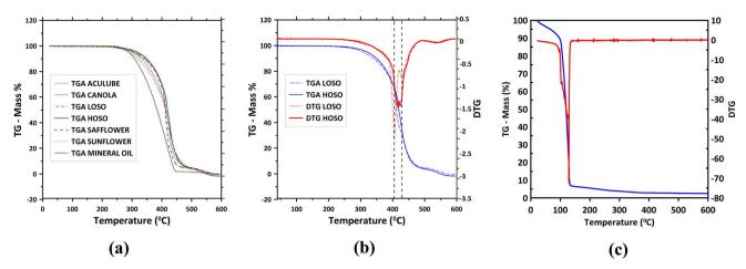
Fig. 5 (a) TGA graphs of various vegetable oils, mineral oil, and LB-2000, (b) combined TGA/DTG graphs of the low oleic and high oleic soybean oils, and (c) TGA and DTG graphs of CEC.
