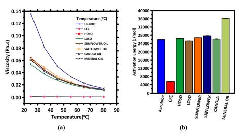
Fig. 4 (a) A graph showing the viscosity-temperature relationship of different vegetable oils compared to CEC, (b): a bar graph comparing the activation energy of various vegetable oils to that of CEC.
