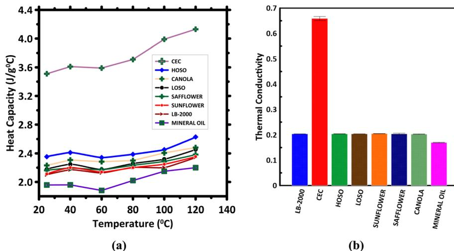
Fig. 6 Graph of: (a) specific heat capacity, and (b) thermal conductivity of the vegetable oils compared with mineral oil, LB-2000 and CEC.
