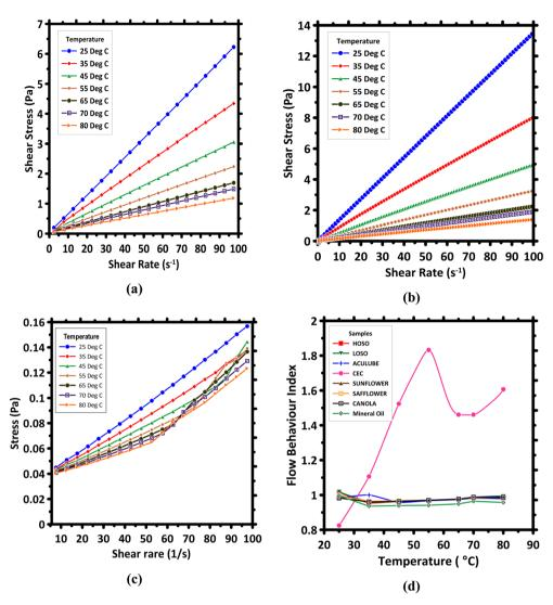
Fig. 3 Temperature-dependent flow behavior of the fluids: (a) flow curves of HOSO as a function of temperature, as a representative of the vegetable oils; (b) flow curve of the mineral oil as a function of temperature; (c) flow curve of CEC as a function of temperature; (d) flow behavior index of CEC compared to the vegetable oils, mineral oil, and LB-2000.
