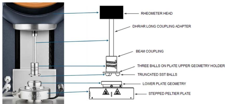
Fig. 1 Schematics of the tribo-rheological setup utilized in the study, in accordance with the instruction manual provided by TA Instruments-Waters LLC.<sup>42</sup>
