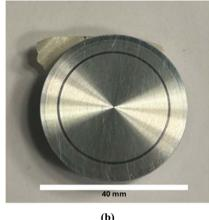
Fig. 8 Wear of the bottom aluminum plate from the tribology tests with: (a) CEC as the lubricant, and (b) HOSO vegetable oil as the lubricant.
