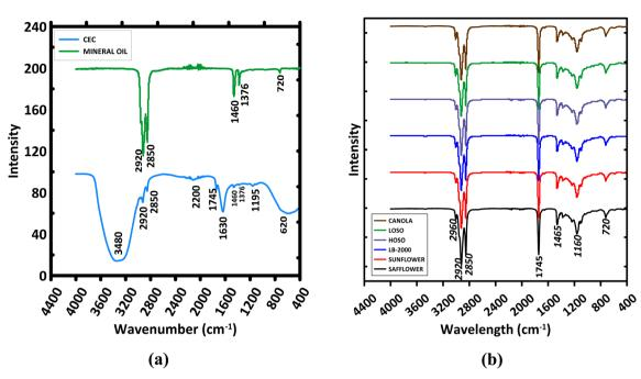
Fig. 2 FTIR spectra of (a) conventional emulsion coolant and mineral oil, (b) the vegetable oils and LB-2000
