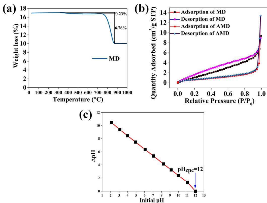
Fig. 5 (a) TGA plot of MD indicating a major weight loss of 6.76% around 1123 K (b)  $\text{N}_2$  adsorption BET plot of AMD used for MB removal (type IV isotherm) (c)  $\text{pH}_{\text{zpc}}$  plot of the adsorbent AMD for the removal of MB ( $\text{pH}_{\text{zpc}} = 12$ ) [0.01 M NaCl from 2 to 12 pH with 0.2 g of AMD for 48 hours at room temperature].
