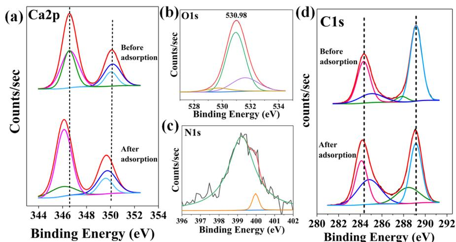
Fig. 9 XPS results indicating (a) Ca 2p spectra before and after adsorption (b) O 1s spectra after adsorption (c) N 1s spectra after adsorption (d) C 1s spectra before and after adsorption.
