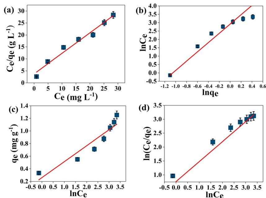
Fig. 8 Adsorption isotherm plots for MB dye removal [initial MB concentration from  $10\text{--}70 \text{ mg L}^{-1}$  at  $1 \text{ g}$  AMD dose for  $135 \text{ min}$  at  $313 \text{ K}$  at  $\text{pH } 6$ ] (a) Langmuir (b) Freundlich (c) Temkin and (d) Redlich–Peterson.
