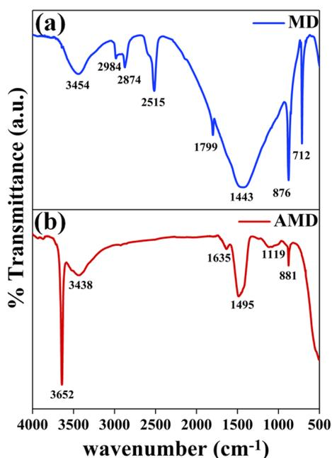
**Fig. 3** FTIR plot of (a) MD and (b) AMD.
