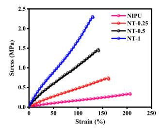
Fig. 5 Stress-strain curves of the NIPU, NT-0.25, NT-0.5, and NT-1 films.
