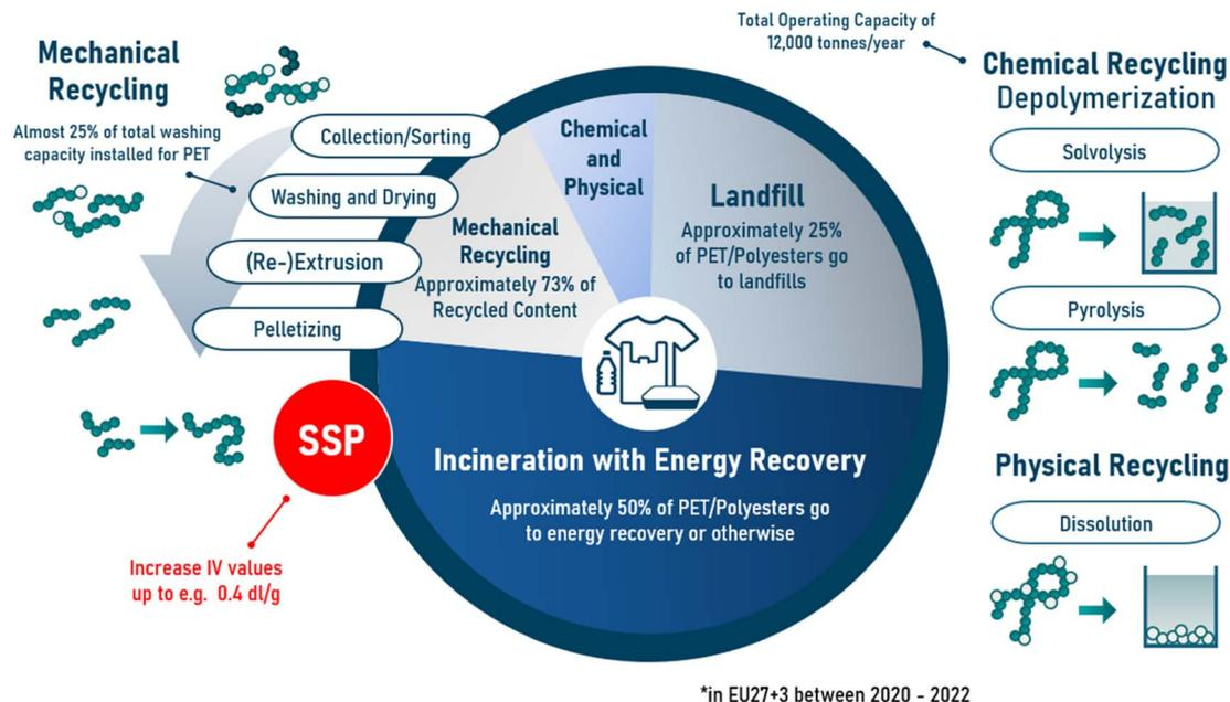
Fig. 1 General principles for PET mechanical recycling via re-processing and PET chemical recycling, complemented with other techniques such as physical recycling via dissolution/precipitation.<sup>8</sup> IV: intrinsic viscosity; SSP: solid-state polymerization.
