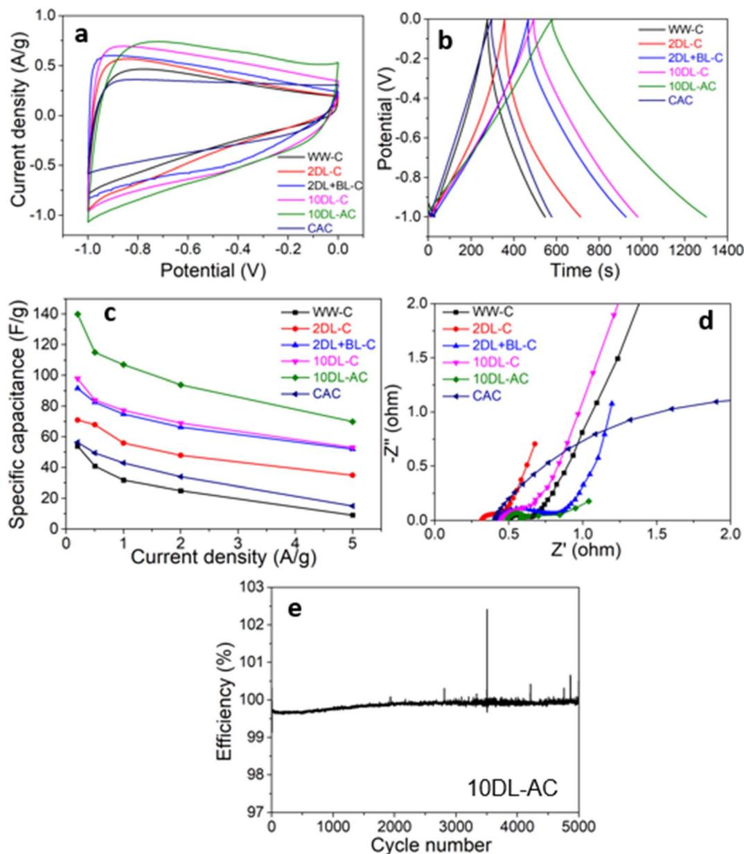
Fig. 6 (a) CV curves at a scan rate of  $5 \text{ mV s}^{-1}$ ; (b) GCD curves at a current density of  $0.2 \text{ A g}^{-1}$ ; (c) specific capacitance as a function of the current densities; (d) Nyquist plots of WW and chemically refined electrodes; and (e) cycling stability of 10DL-AC electrodes in 6 M KOH in a three-electrode system.
