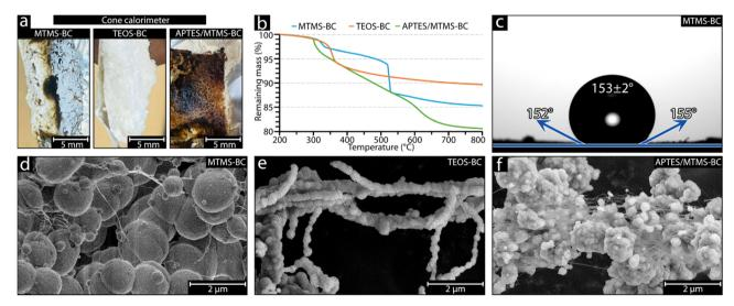
Fig. 6 The various aerogels after cone calorimetry tests (4 min exposure to 618 °C) (a), thermal degradation of the aerogels between 200 and 800 °C (b), and the obtained water contact angle (c). The MTMS-BC, TEOS-BC, and APTES/MTMS-BC aerogel morphology after exposure to 800 °C is shown in (d), (e), and (f) respectively.
