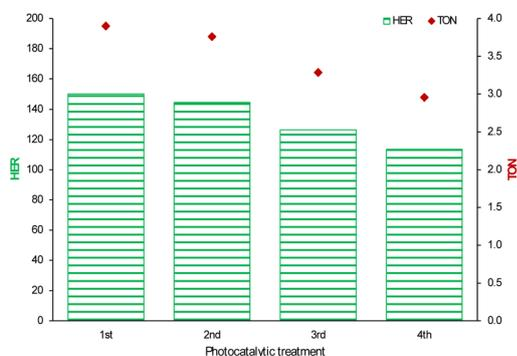
Fig. 6 Reusability of the g-C<sub>3</sub>N<sub>4</sub> catalyst in raw wastewater under simulated solar light ( $n = 2$ ): HER (y-axis on the left), TON (y-axis on the right).
