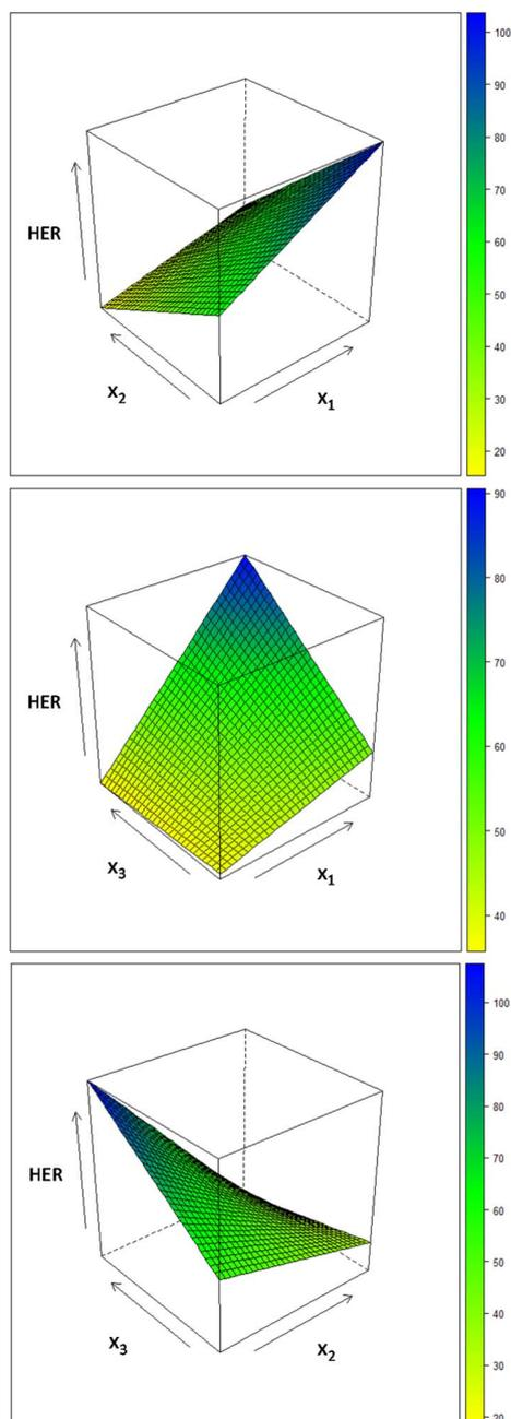
Fig. 5 Response surfaces obtained by CAT from the experimental results of  $\text{H}_2$  production from the wastewater.
