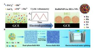
Fig. 10 Fabrication of HEOs through the DES electrodeposition process. (A) Illustration of the programmed electrodeposition method for the preparation of RuRhPdPtAu HEA-NPs. Reprinted with permission from copyright@ Royal Society of Chemistry, 2023.<sup>129</sup>. (B) Process outline for electrochemical dealloying in ChCl-TU DES of FeCo-NiCrMo HEA. Reprinted with permission from copyright@ American Chemical Society, 2023.<sup>130</sup>
