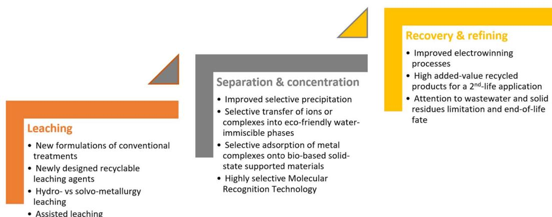
Fig. 8 Innovative chemical approaches for metal recovery of e-waste.
