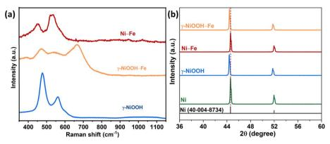
Fig. 1 (a) Raman spectra of  $\gamma$ -NiOOH,  $\gamma$ -NiOOH–Fe and Ni–Fe catalysts; (b) XRD patterns of Ni-foam after acid washing,  $\gamma$ -NiOOH, Ni–Fe, and  $\gamma$ -NiOOH–Fe.
