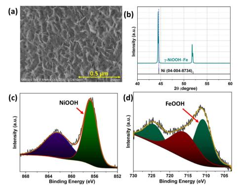
Fig. 6 (a) FE-SEM image, (b) XRD pattern, and (c) and (d) XPS Ni 2p peaks and Fe 2p peaks of  $\gamma$ -NiOOH-Fe respectively, after the electrolysis at 80 °C.
