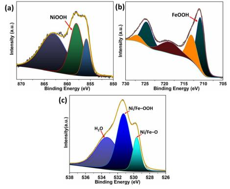
Fig. 2 Deconvoluted XPS spectra (a) Ni 2p, (b) Fe 2p and (c) O 1s spectra of γ-NiOOH-Fe.
