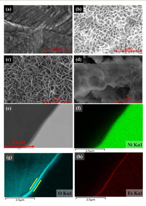
Fig. 3 FE-SEM images of (a) the bare Ni foam surface, (b) Ni foam surface after oxidation ( $\gamma$ -NiOOH), (c)  $\gamma$ -NiOOH–Fe and (d) Ni–Fe. (e) Cross-sectional SEM-EDX image of  $\gamma$ -NiOOH–Fe, and EDX mapping of (f) nickel, (g) oxygen, and (h) iron.
