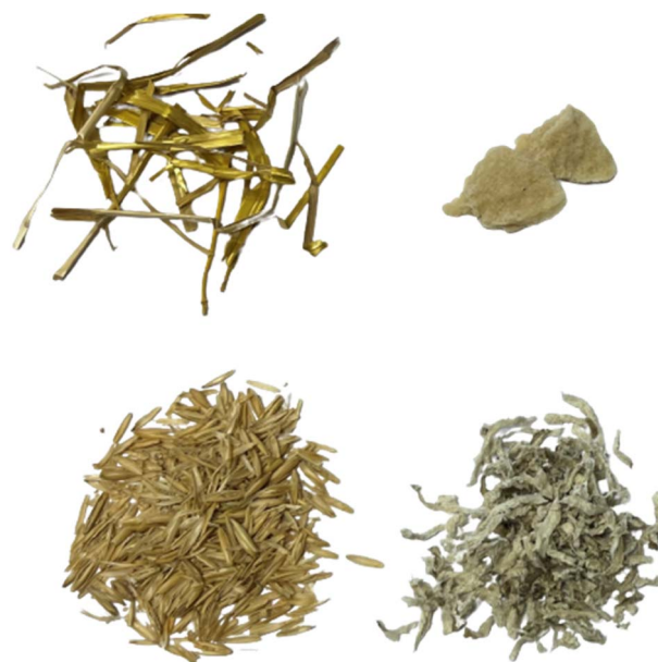
Fig. 1 Raw materials before pulping from top left: wheat straws, potato pulp, oat husks and pressed sugar beets.
