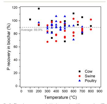
Fig. 5 Phosphorus recovery in biochars produced from cow (n=15), swine (n=25), and poultry manure (n=25). The average value of 89.9% is calculated over all temperatures and manure types. Values are based on data from various sources. 47–50.56.57.59.65.68–70.124
