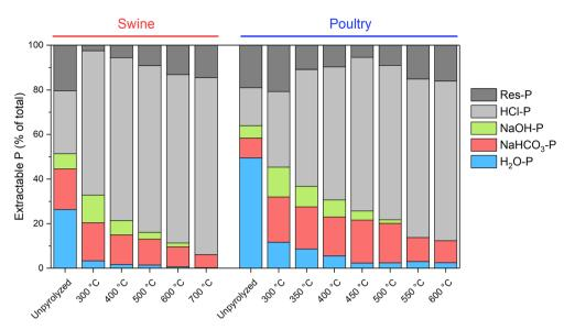
Fig. 9 Sequential fractionation of biochars produced at different temperatures from swine manure (data taken from Jiang et al.<sup>57</sup>) and poultry litter (data taken from Li et al.112). Increasing the pyrolysis temperature decreases the H<sub>2</sub>O-P fraction and increases the HCl-P fraction.
