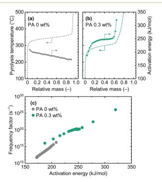
Fig. 2 TGA of cellulose loaded with 0 and 0.3 wt% of PA. Pyrolysis curves (temperature vs. relative mass) obtained by TGA at different heating rates (5, 10, 15, and 20 °C min<sup>-1</sup>) were analyzed with DAEM model.35 Pyrolysis curves in (a) and (b) were obtained at 10 °C minand shown as the representative results.
