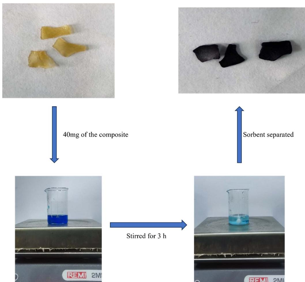
Scheme 2 Representative method for adsorption of MB dye solution using chitosan–IL composites.
