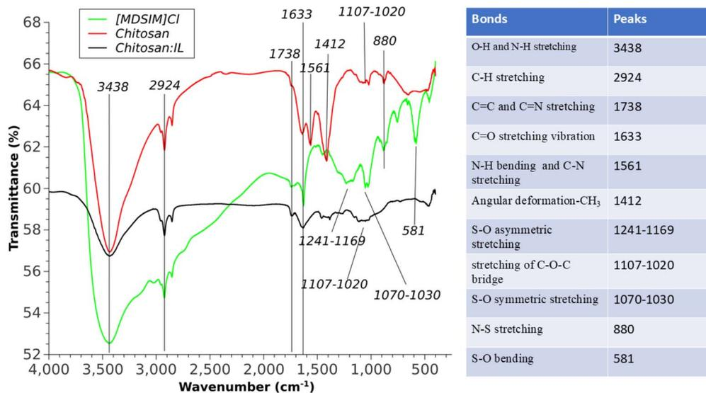
Fig. 2 FTIR spectra of chitosan, chitosan-IL and [Mdsim]Cl.
