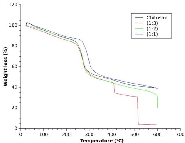
Fig. 7 TGA profile of different chitosan–IL composites.
