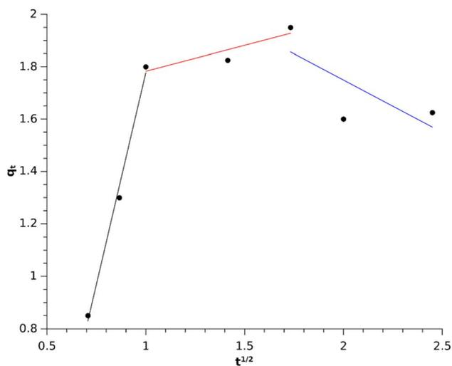
Fig. 13 Intra-particle diffusion model for MB adsorption.
