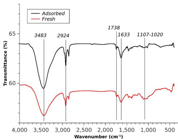
Fig. 16 FTIR spectra of fresh and adsorbed composites.
