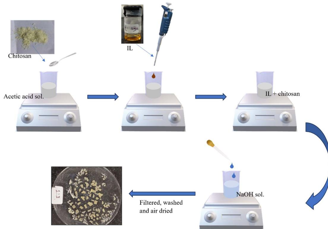
Scheme 1 Representative procedure for preparation of chitosan-IL composites.
