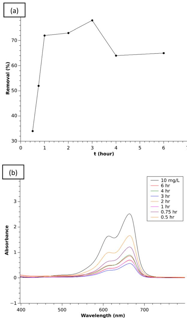
Fig. 11 (a) Effect of time on the adsorption behavior of the 1 : 3 composite and (b) UV plots for adsorption of MB solution (10 mg L<sup>-1</sup>) during 6 h adsorption time using the 1 : 3 composite.
