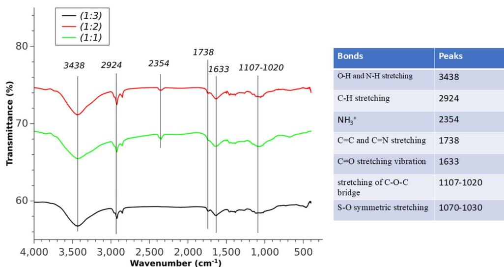
Fig. 3 Comparative FT-IR spectra of chitosan-IL composites.
