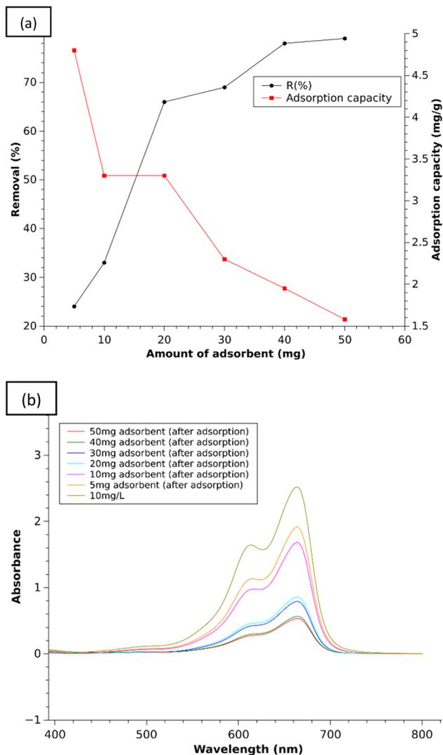
Fig. 10 (a) % Removal efficiency and adsorption capacity of the 1 : 3 composite with increasing amount and (b) UV plots of MB solution (10 mg L<sup>-1</sup>) after adsorption with increasing amount of the 1 : 3 composite.
