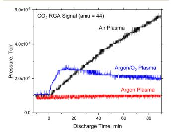
Fig. 5 The comparison of RGA CO<sub>2</sub> signals (amu = 44) under argon, 50% oxygen (balanced by Ar) and air plasmas with the presence of CaCO<sub>3</sub> powders.
