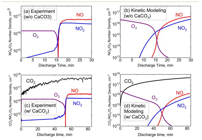
Fig. 2 A comparison between experimental measurements (a and c) and kinetic modelling (b and d) for the case with and without CaCO<sub>3</sub> powders. Fitting parameters:  $n_{\rm O}=1.4\times10^{11}$  cm<sup>-3</sup>.  $T_{\rm V}^0=7500$  K.  $\tau_{\rm V}=1.2\times10^3$  s for (b).  $\tau_{\rm V}=5.0\times10^3$  s for (d).
