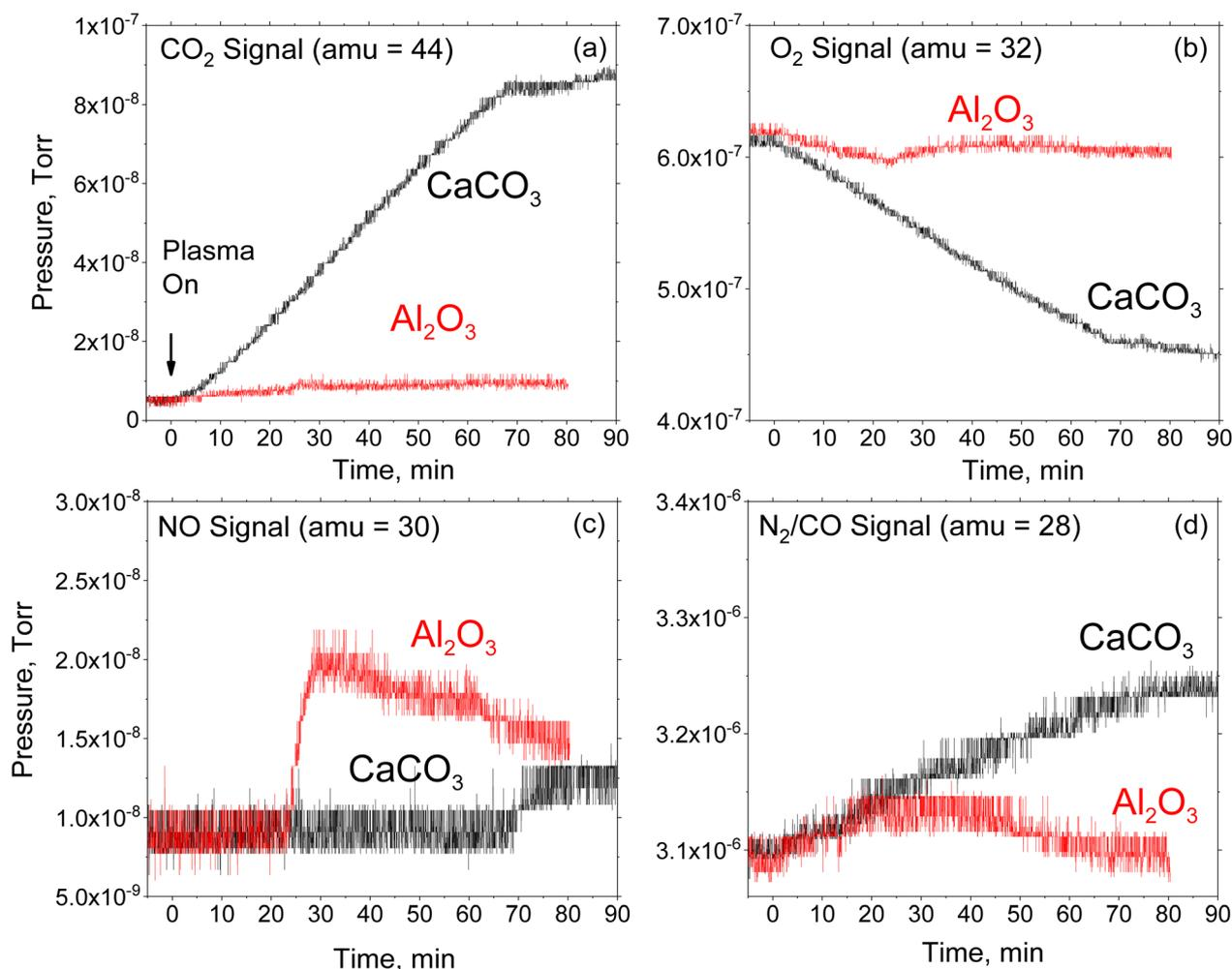
**Fig. 3** Time dynamics of (a)  $\text{CO}_2$ , (b)  $\text{O}_2$ , (c)  $\text{NO}$ , and (d)  $\text{N}_2/\text{CO}$  in the gas phase detected by RGA during the plasma-assisted  $\text{CO}_2$  desorption. Data were obtained for loading  $\text{CaCO}_3$  particles or  $\text{Al}_2\text{O}_3$  particles (10 g). Reaction conditions: 1 atm, 300 K, total flow rate 10 sccm.
