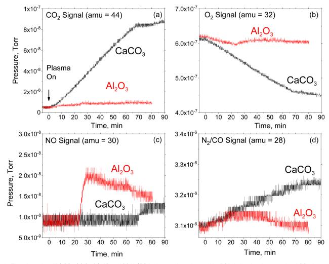
Fig. 3 Time dynamics of (a) CO<sub>2</sub>, (b) O<sub>2</sub>, (c) NO, and (d) N<sub>2</sub>/CO in the gas phase detected by RGA during the plasma-assisted CO<sub>2</sub> desorption. Data were obtained for loading CaCO<sub>3</sub> particles or Al<sub>2</sub>O<sub>3</sub> particles (10 g). Reaction conditions: 1 atm, 300 K, total flow rate 10 sccm.
