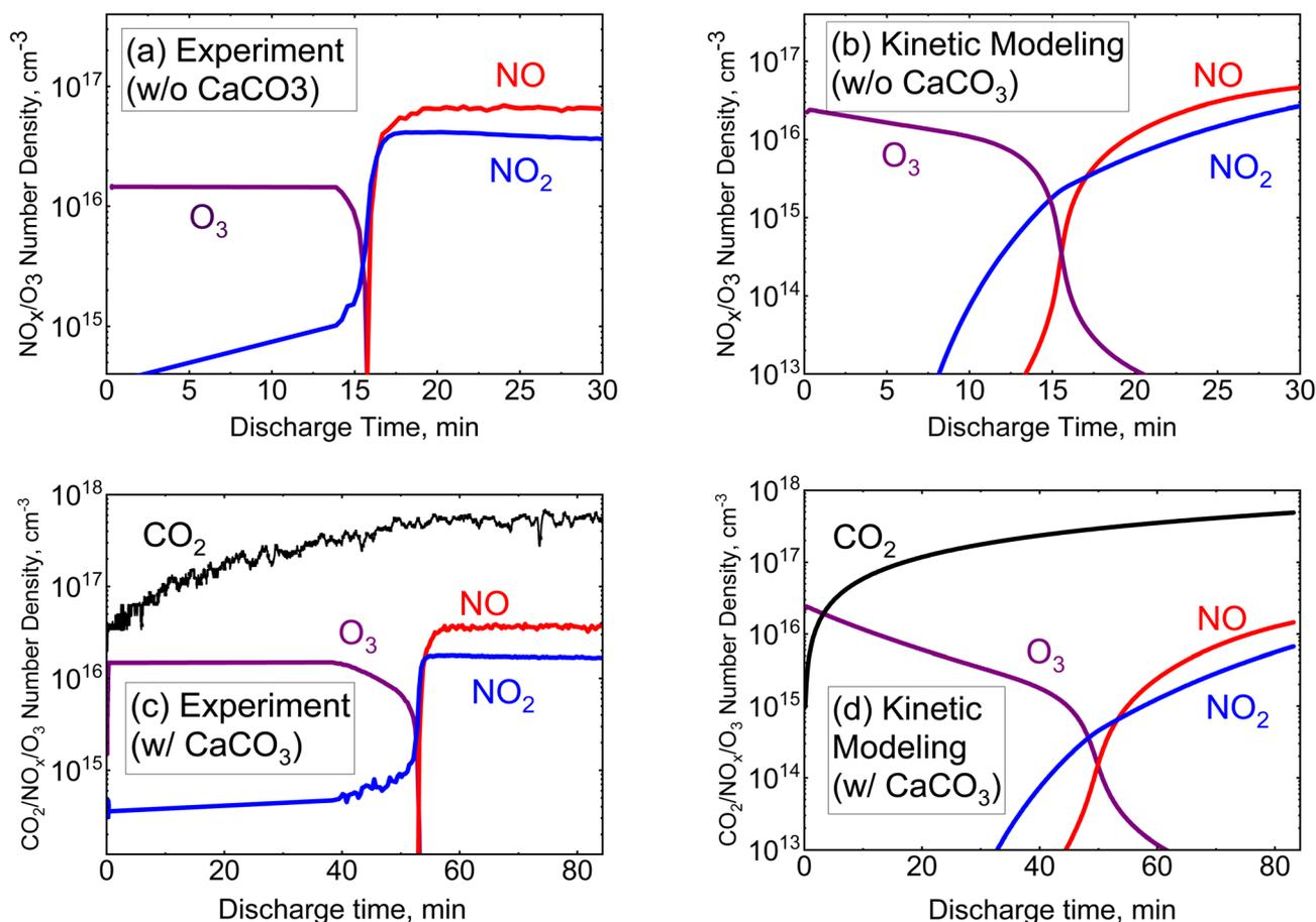
**Fig. 2** A comparison between experimental measurements (a and c) and kinetic modelling (b and d) for the case with and without  $\text{CaCO}_3$  powders. Fitting parameters:  $n_{\text{O}} = 1.4 \times 10^{11} \text{ cm}^{-3}$ ,  $T_{\text{v}}^0 = 7500$  K,  $\tau_{\text{v}} = 1.2 \times 10^3$  s for (b),  $\tau_{\text{v}} = 5.0 \times 10^3$  s for (d).
