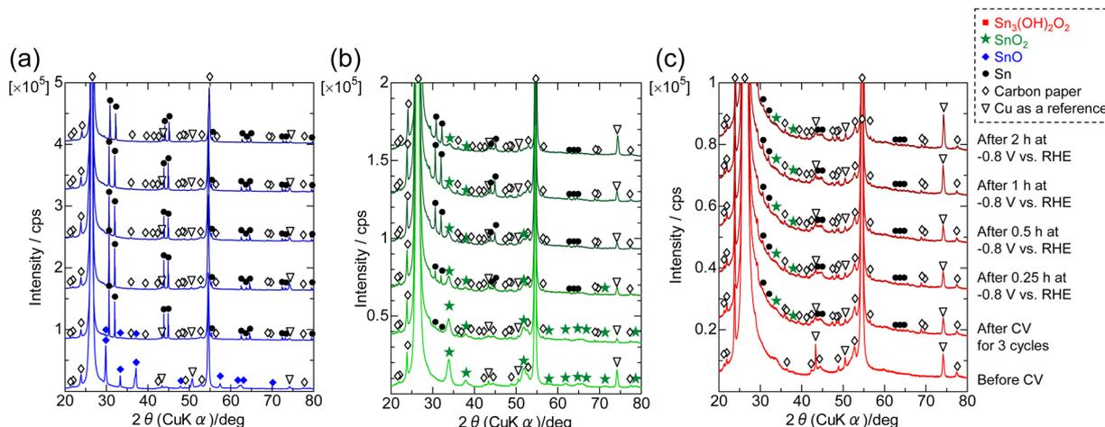
Fig. 3 XRD patterns of (a) ST-SNO, (b) SG-SNO and (c) P-SNO loaded on carbon paper electrodes before and after CV between 0.5 and  $-1.2$  V vs. RHE with  $10 \text{ mV s}^{-1}$  for 3 cycles, and constant potential measurements at  $-0.8$  V vs. RHE for 0–2 h in  $\text{CO}_2$  saturated  $\text{NaHCO}_3$  aqueous solution.
