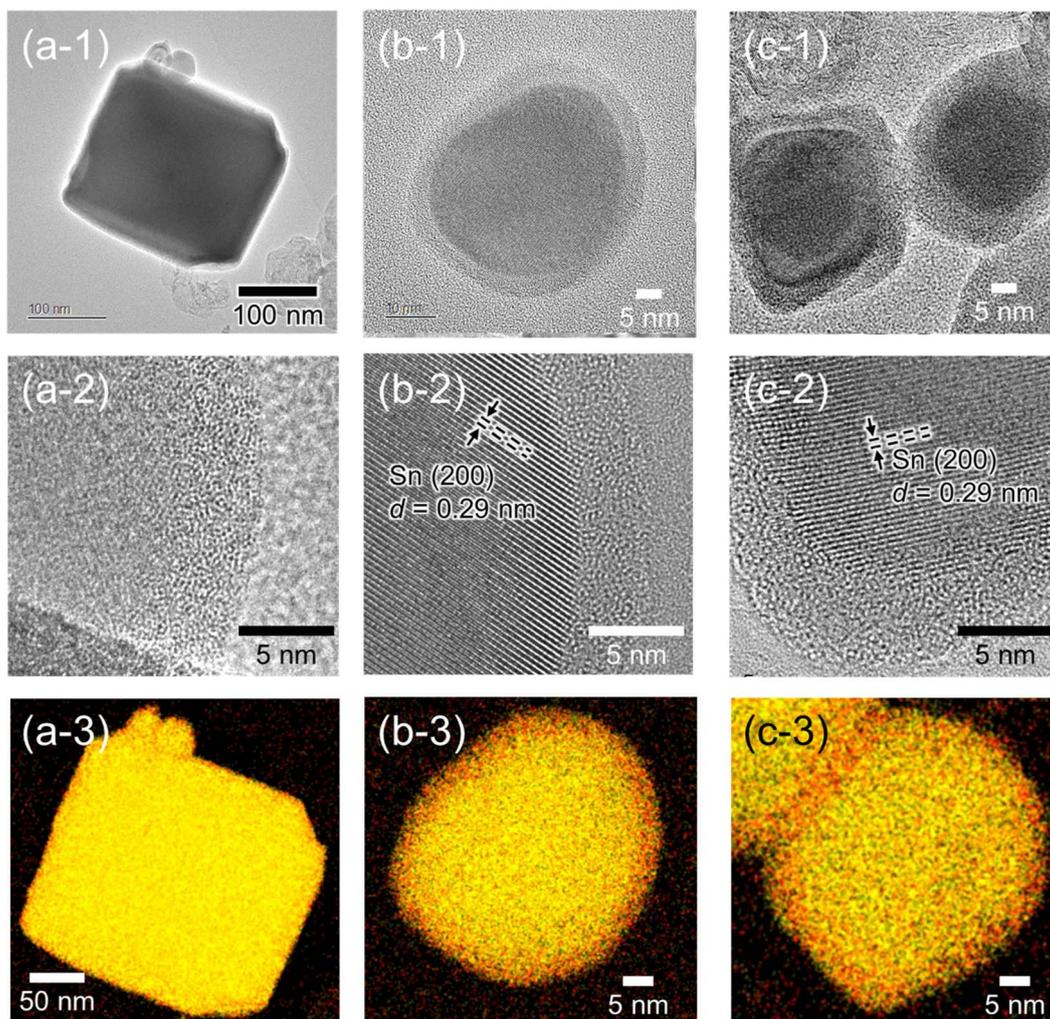
Fig. 5 (1 and 2) HR-TEM images and (3) EDS mappings of (a) ST-SNO, (b) SG-SNO and (c) P-SNO/carbon paper electrodes after constant potential measurements at  $-0.8$  V vs. RHE for 0–2 h in  $\text{CO}_2$  saturated  $\text{NaHCO}_3$  aqueous solution.
