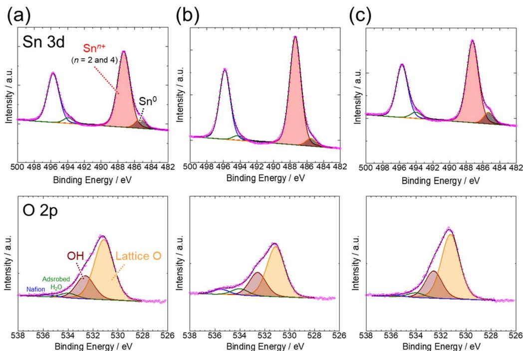
Fig. 6 XPS spectra of Sn3d and O2p of (a) ST-SNO, (b) SG-SNO and (c) P-SNO/carbon paper electrodes after constant potential measurements at  $-0.8$  V vs. RHE for 0–2 h in  $\text{CO}_2$  saturated  $\text{NaHCO}_3$  aqueous solution.
