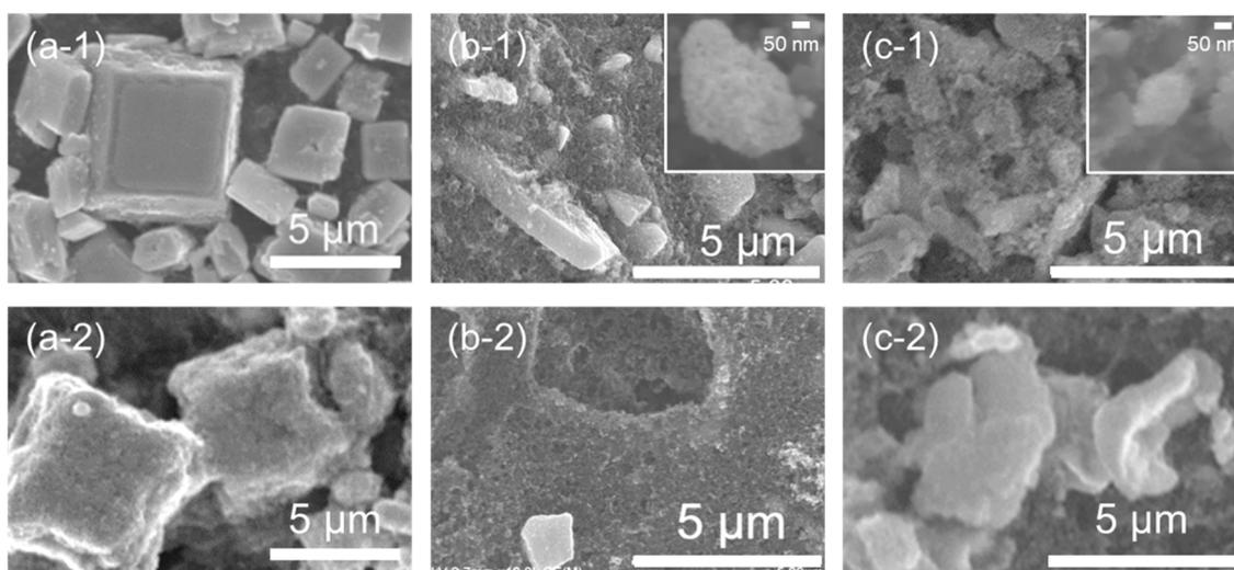
Fig. 4 SEM images of (a) ST-SNO, (b) SG-SNO and (c) P-SNO/carbon paper electrodes (1) before and (2) after constant potential measurements at  $-0.8$  V vs. RHE for 2 h in  $\text{CO}_2$  saturated  $\text{NaHCO}_3$  aqueous solution. Inset figures in (b-1) and (c-1) are the enlarged figures of SG-SNO and P-SNO, respectively, before the reaction.
